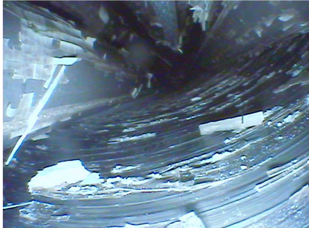
bundle elevation 650 mm: spalled oxide scales at shroud and cladding
