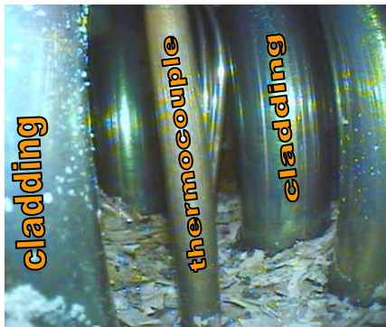
-400mm: spalled oxide scales as debris at the bundle bottom
