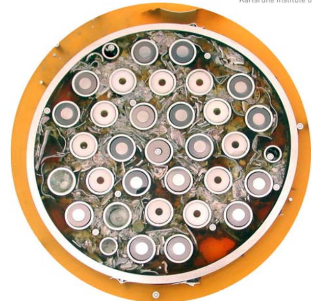
Q12: rubble on spacer grid consists of spalled cladding scales and fragments of partially oxidized cladding
