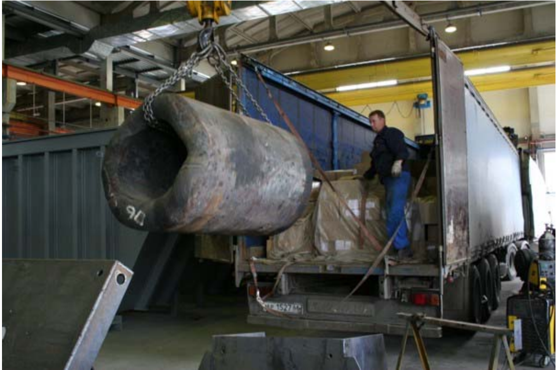
Fig. 3.3.5 – unloading of the billet from the 15Kh2NMFA steel
