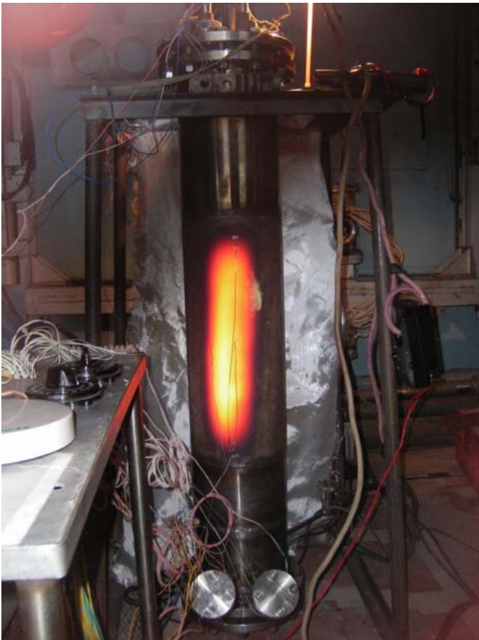
Fig. 3.4.7 – Fragments of the heater element testing
