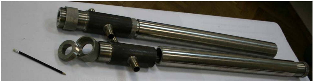
Fig. 3.4.4 – The upper part of the heater current-carrying arrangement
