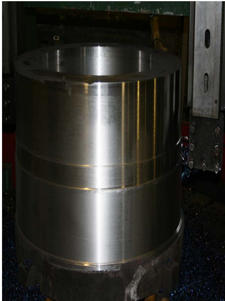
Fig. 3.3.7 – Preparation and machining of the vessel models from the billet
