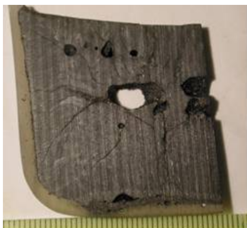
Fig. 2.7- Ingot axial section
