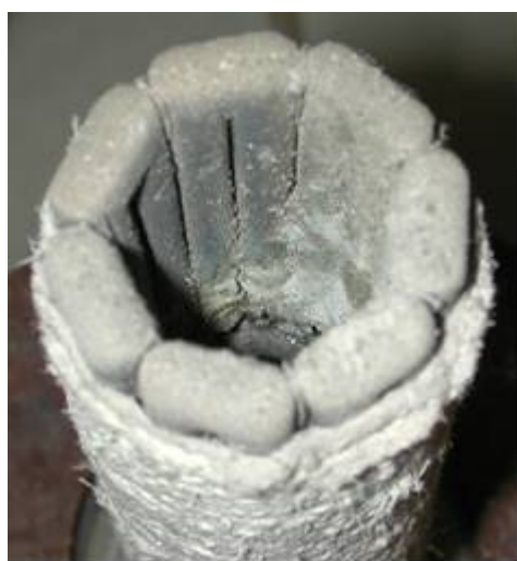
Fig. 2.43- Crucible after PRS10
