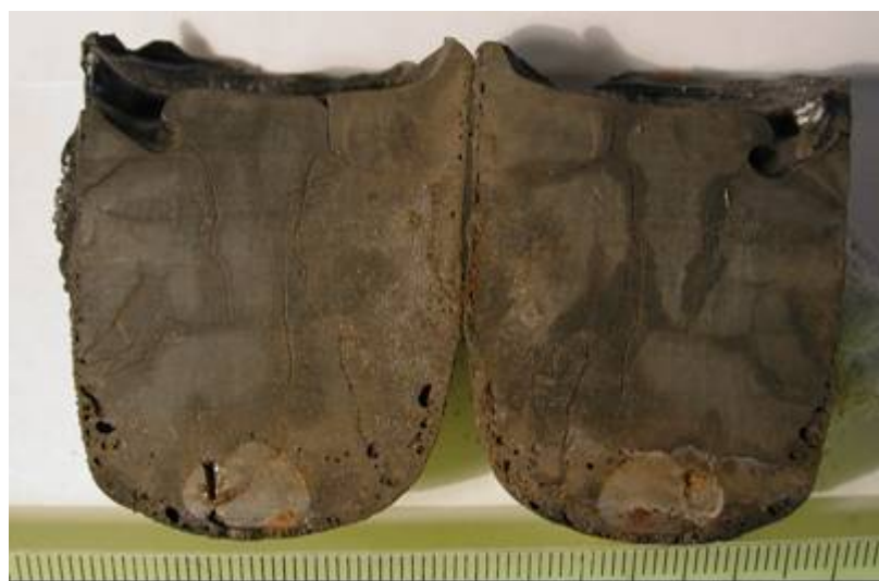
Fig. 3.6- Axial section of PRS13 ingot
