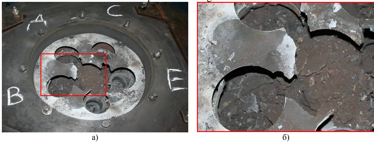
Figure 159 – RPV model with solidified melt after plasmatrons dismantling
