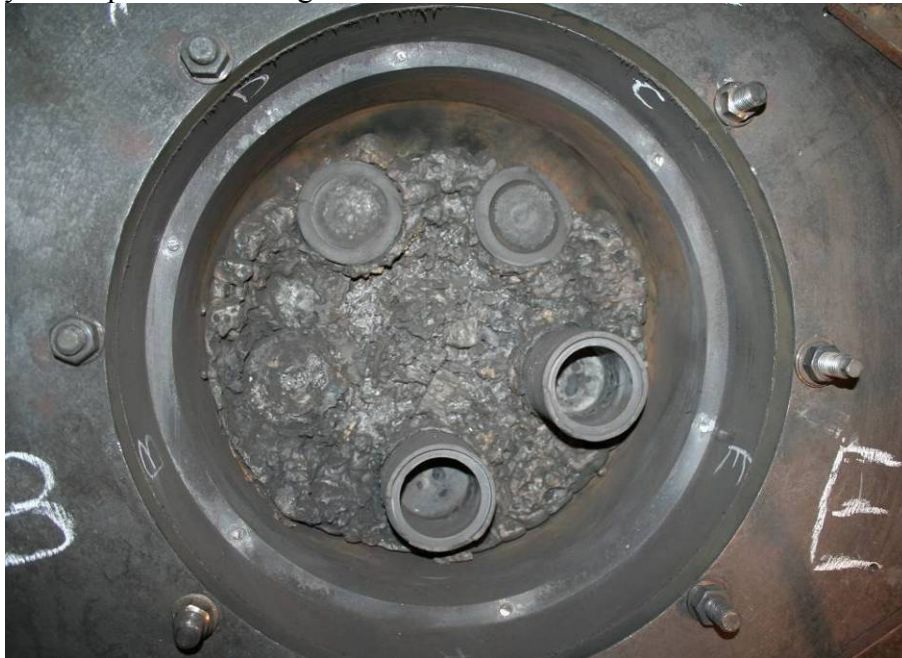
Figure 160 – The vessel model with the melt after removal of the fragments layer
