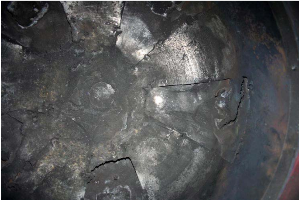
Figure 145 – The vessel model surface after corium removal
