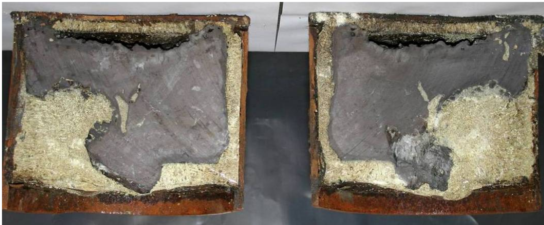
Figure 34 – Longitudinal section of the corium ingot
