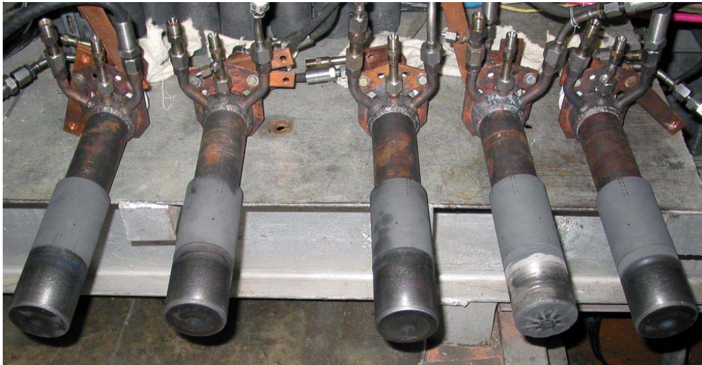
Figure 90 – Coaxial plasmatrons before their installation in the experimental section
