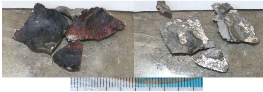
Figure 169 – Appearance of the crust surface (samples OI-5-2) from the vessel model side (on the left) and the break surface from the ingot side (on the right)
