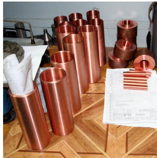
f) Copper parts of the coaxial plasmatrons
