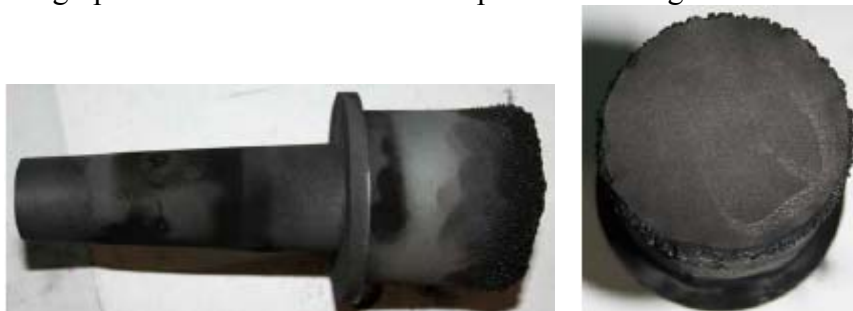
Figure 69 – Graphite nozzle of the internal electrode after the test
