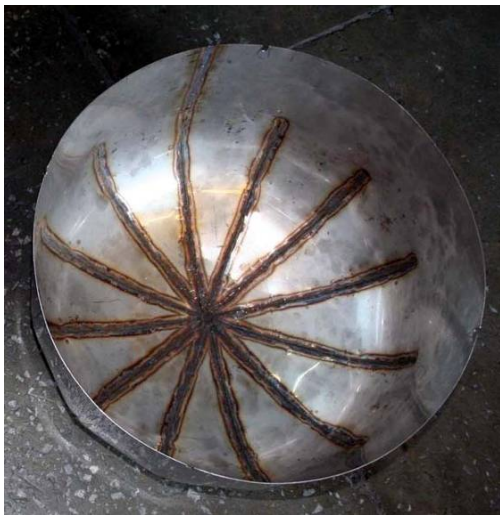
e) Steel shield of the insulation
