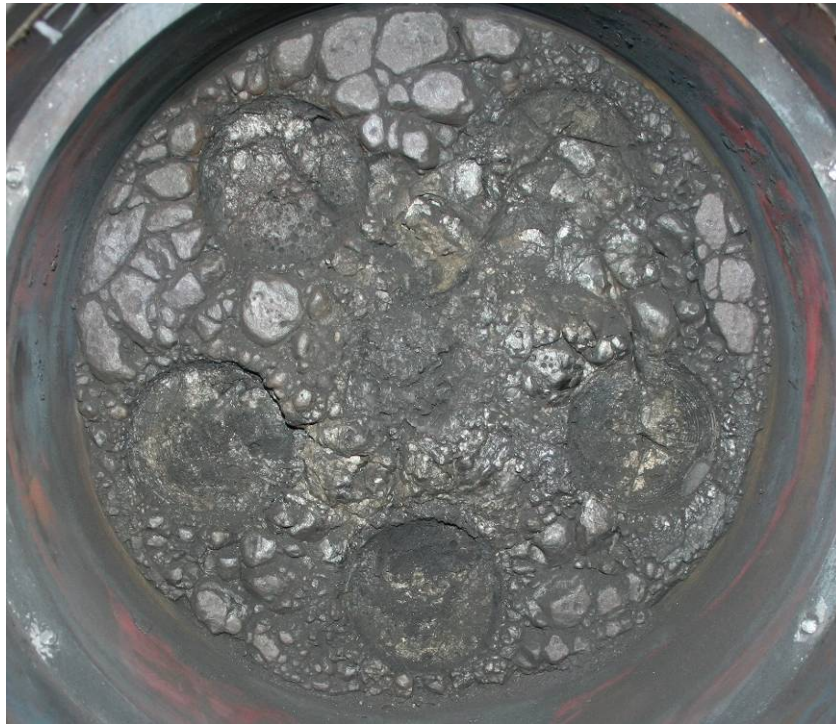
Figure 166 – The appearance of the corium ingot surface after removal of the disconnected fragments The diagram of the ingot fragments sampling is represented in Figure 167.
