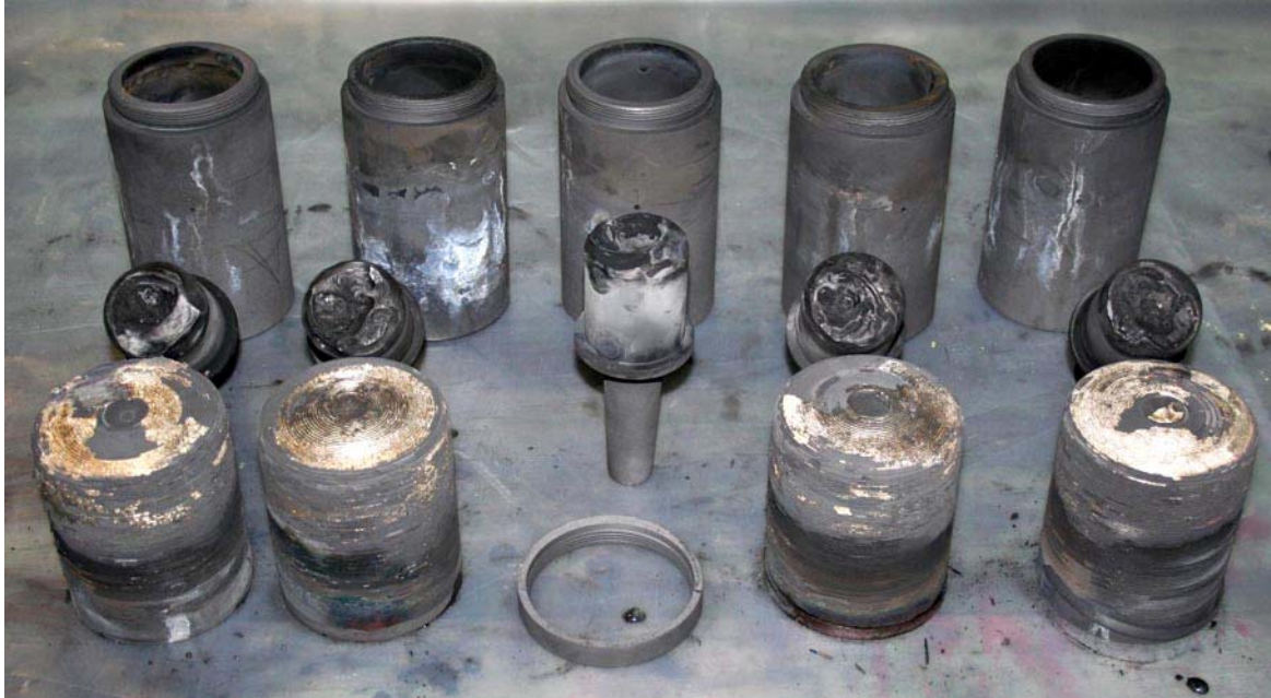
Figure 96 – Condition of the plasmatrons electrode nozzles
