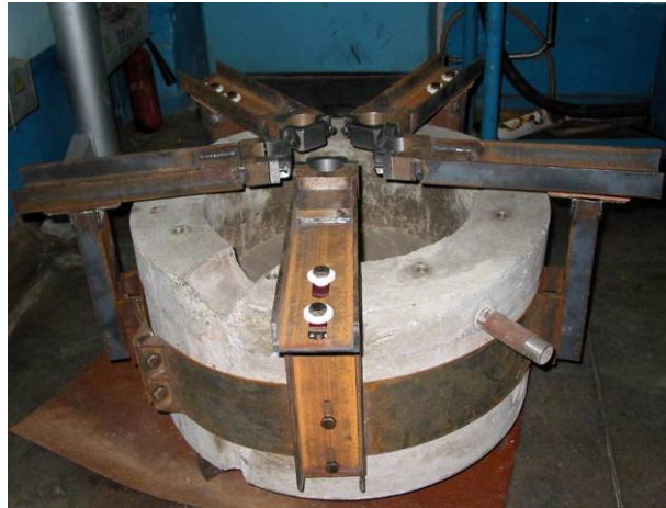
b) Concrete base of the experimental section with holders for the plasmatrons
