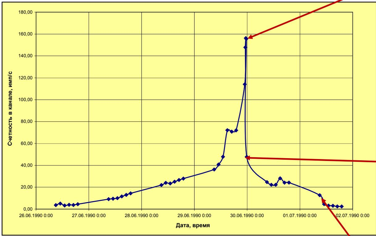
**a) Neutron sensors located in neighboring premises 304/3, fixed consequent increase in flux density of neutron leak (via 1-m concrete wall) from premises 305/2 in more than 60 times (Fig. 9) – system took conditions of multiplying medium with positive reactivity.**
