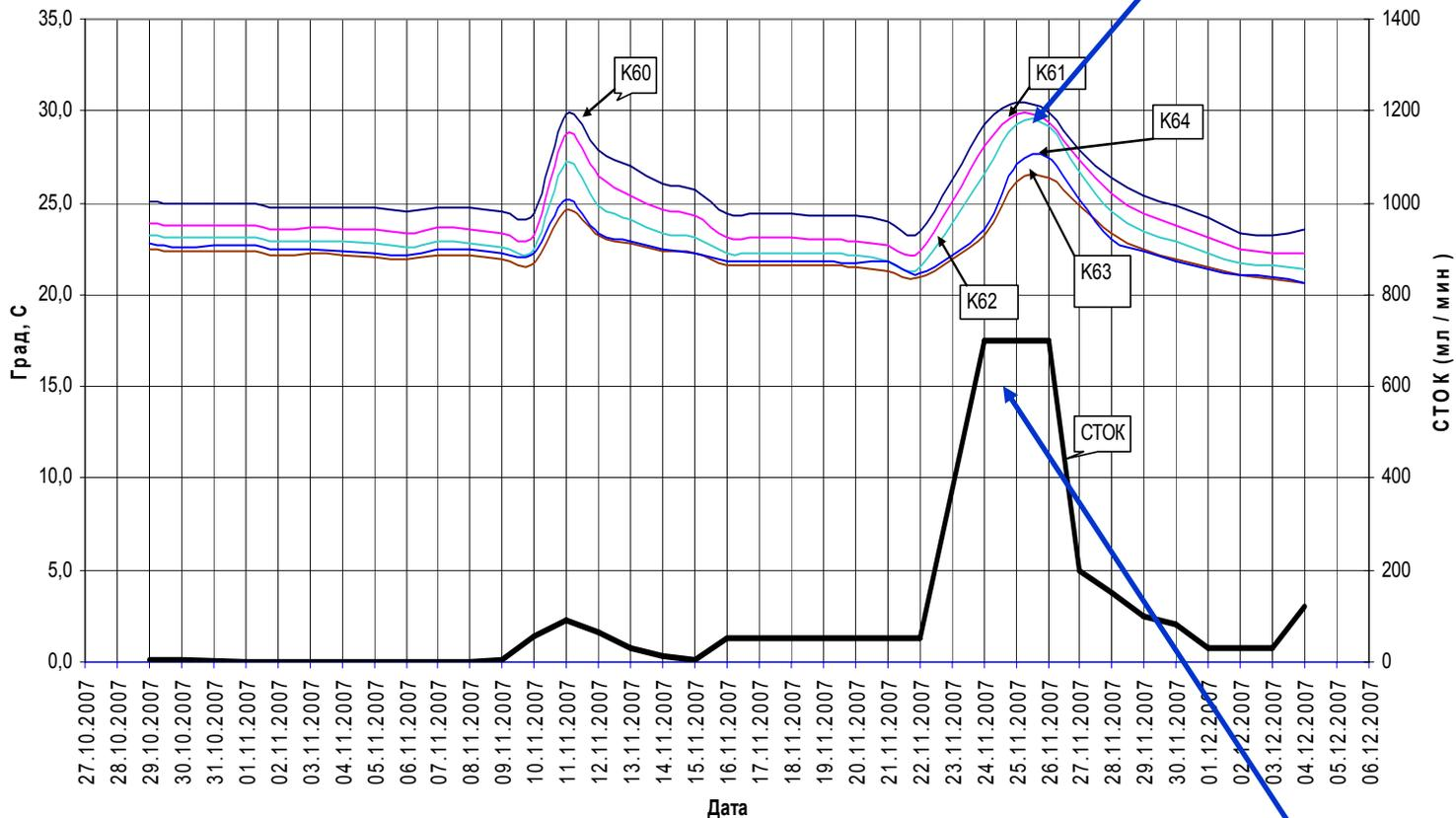
temperature jump on borehole 3.9.K
