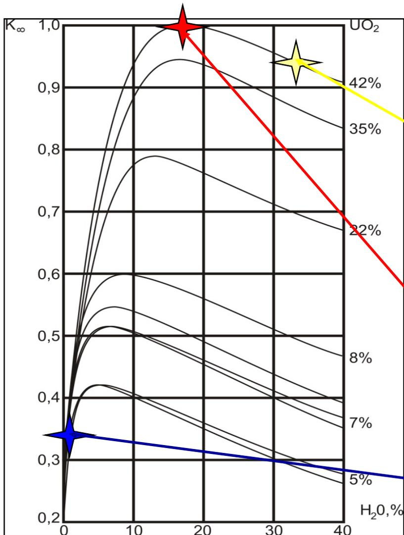
**Estimates of effective neutron multiplying factor (Fig. 10) for medium with low-enriched uranium in composition  $\text{UO}_2 + \text{SiO}_2 + \text{H}_2\text{O}$  demonstrated as regards:**
