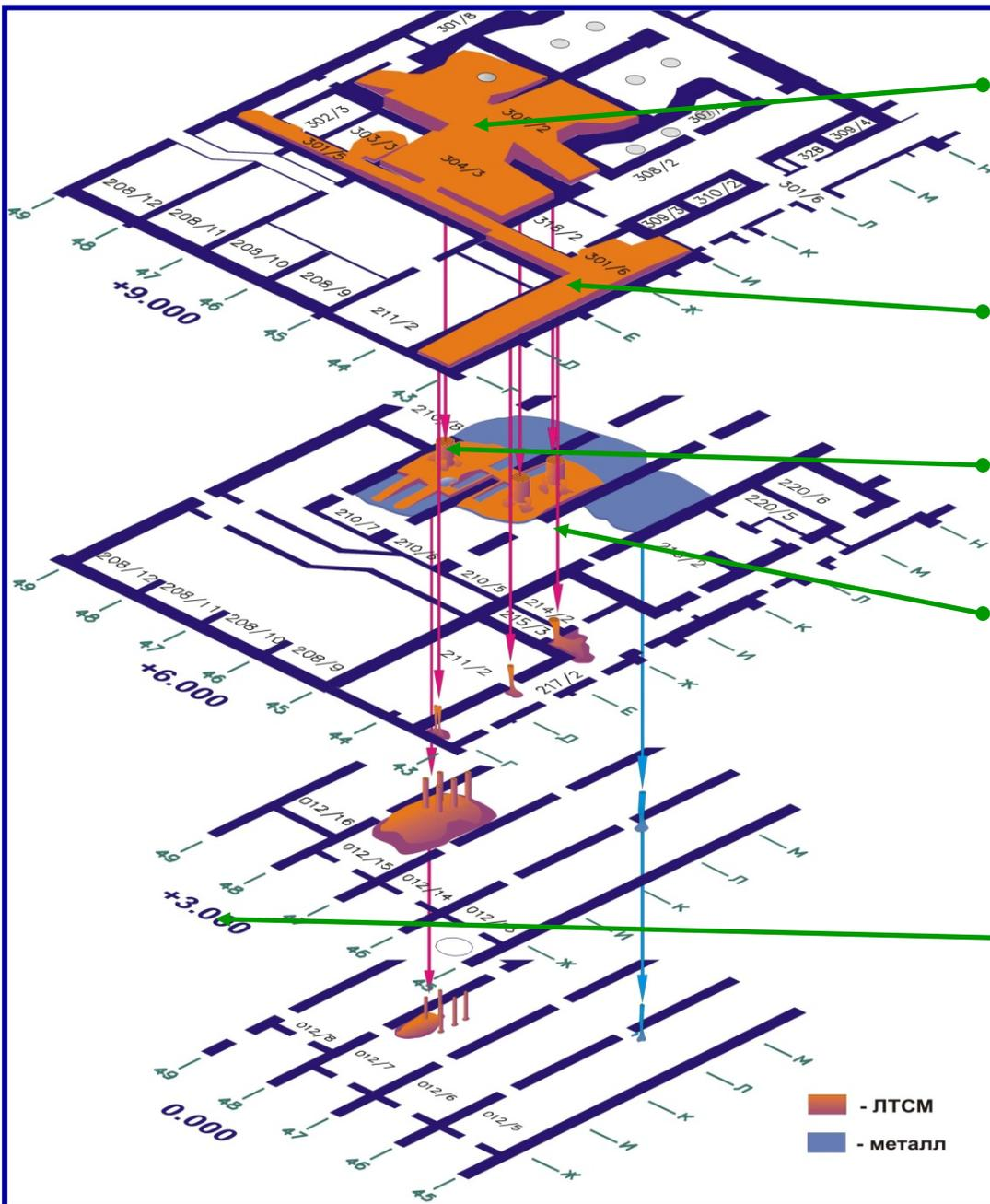
Main process of lava-like fuel containing materials (LTCM) origination occurred in premises 305/2. Further, LTCM spread by three basic flows
