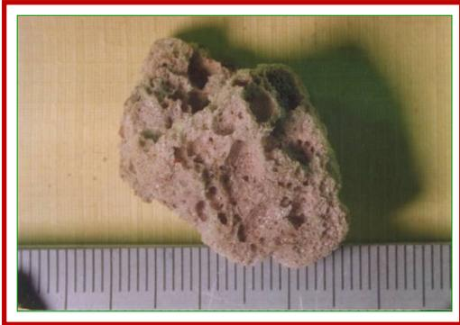
**LTCM cluster on first floor of pressure suppression pool (porous ceramics)**
