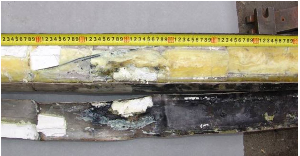
Fig. 1. External appearance of the thermal insulation housing inner surface at the level of 700-1300 mm.
