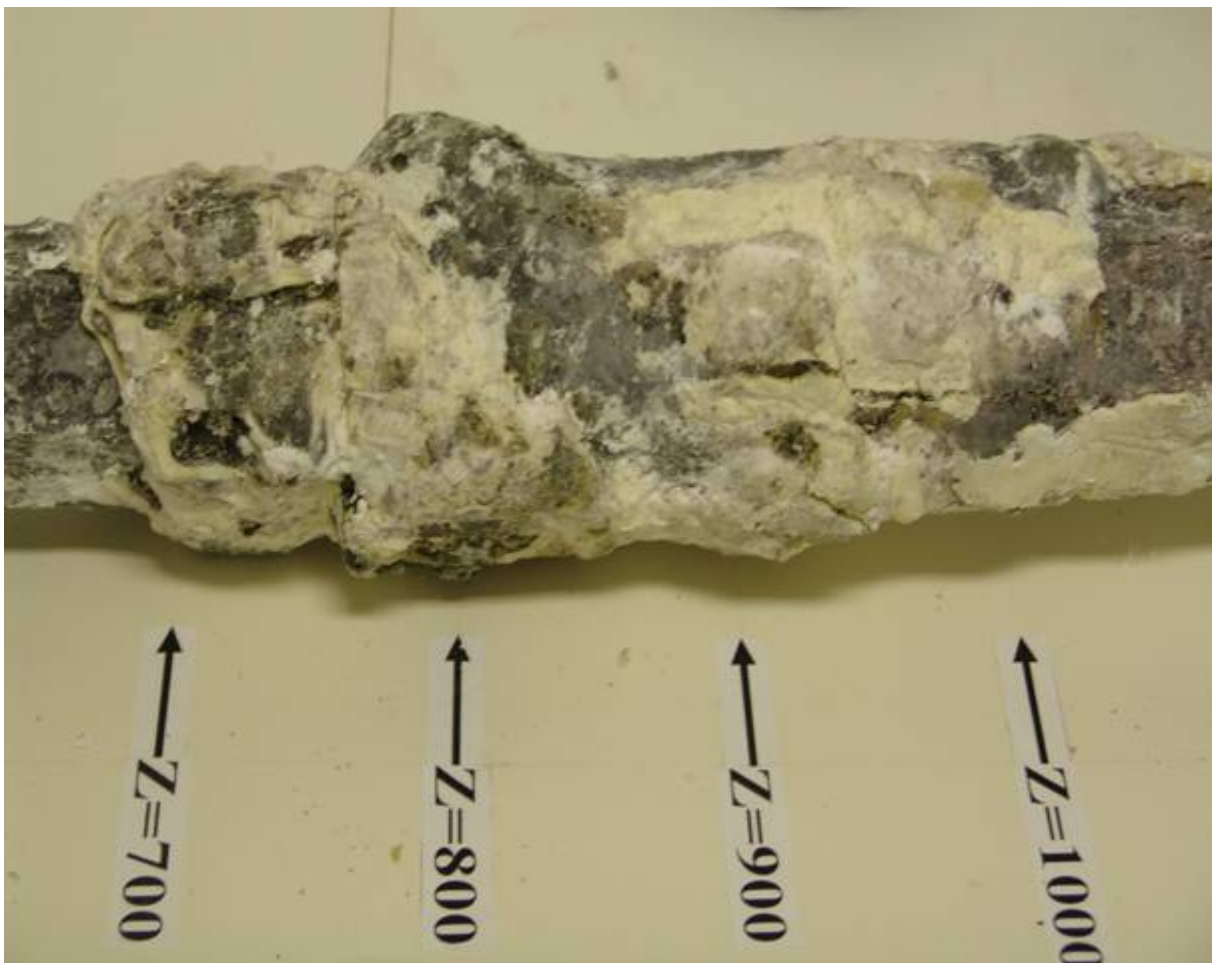
Fig. 2. External appearance of the shroud after the tests (level 700 – 1000 mm, 90° – 120°).
