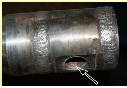
The loss of the integrity occurred because of an internal engineering flaw of the welded seam connecting the two parts of the electrical conductor made of copper and the stainless steel
