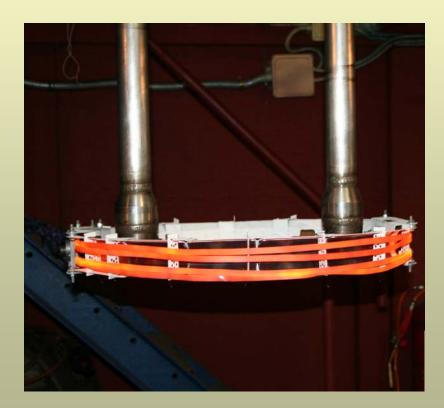
•3. Task "C": The preparation of the scale experiment on the high-temperature heat-up and creep deformation of the vessel model (6)
