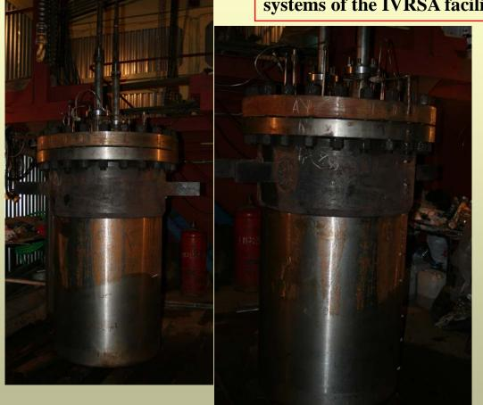
Test for leak integrity of the scale model and auxiliary systems of the IVRSA facility
