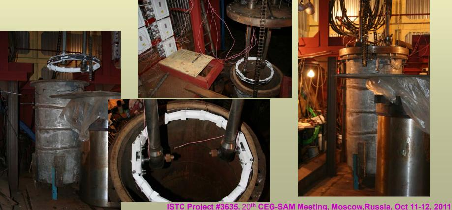
•3. Task "C": The preparation of the scale experiment on the high-temperature heat-up and creep deformation of the vessel model (7)
