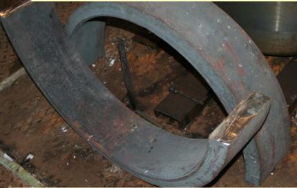
With the purpose of identification of high-temperature mechanical characteristics of the steel the vessel scale model is made of it was decided to make a control batch of samples from the test and to conduct a creep test of this steel.
