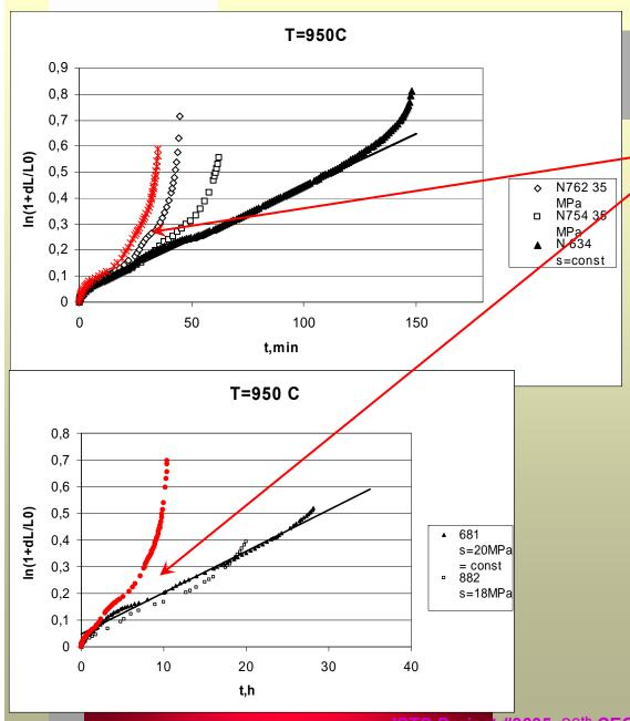
3) in the range of 900-950 C creep characteristics of the two types of steel is almost the same.
