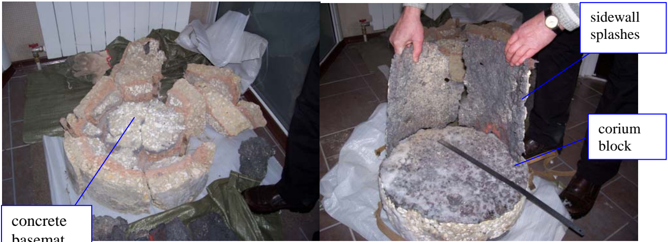
Figure 6a: concrete basemat after disassembly
