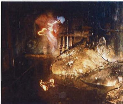
Figure 5.9. – Room #217/2. “Elephant’s foot” and a “Stalactite”
