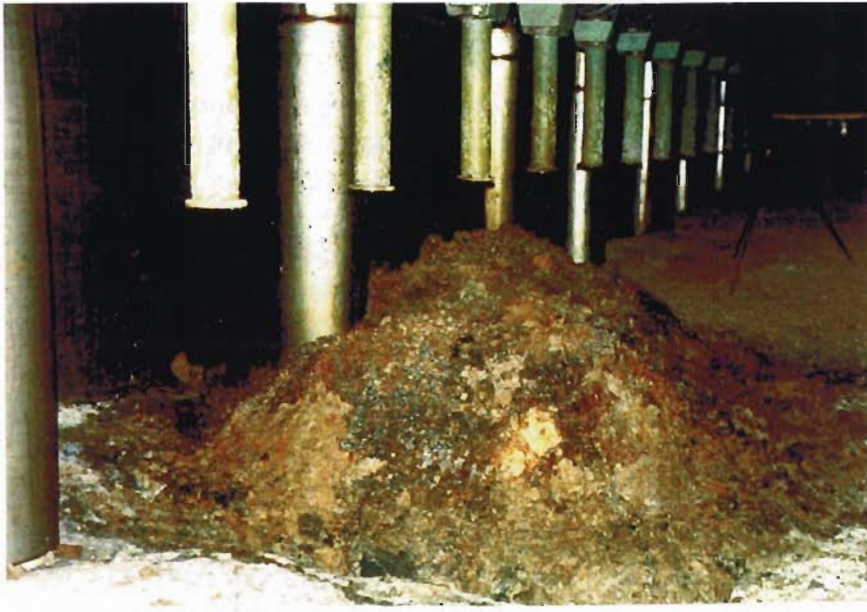
Fig.5.23. LFCM “pile” on the first floor of PSP, Room #012/7
