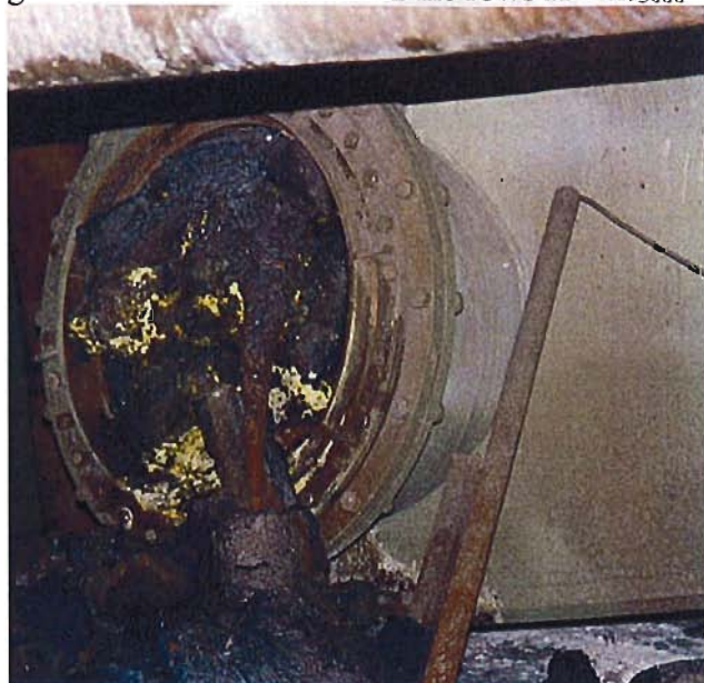
Fig.5.19. Canary-colored spots – new formations on LFCM surface (Room #210/6)
