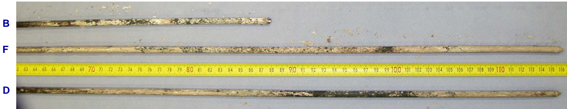
corner rods D, F, B after pre-test: spalling of the outer skin of oxide layer.
