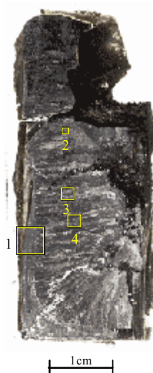
Fig. 2.11. Axial section of CORD 17 ingot with studied segments
