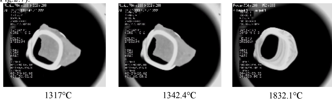
Fig. 3.3. View of sample in the iridium holder during VPA in the Galakhov microfurnace
