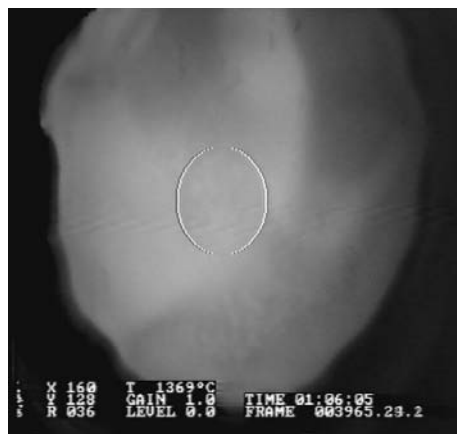
Fig. 7. Video image of the melt surface during the liquidus temperature measurements
