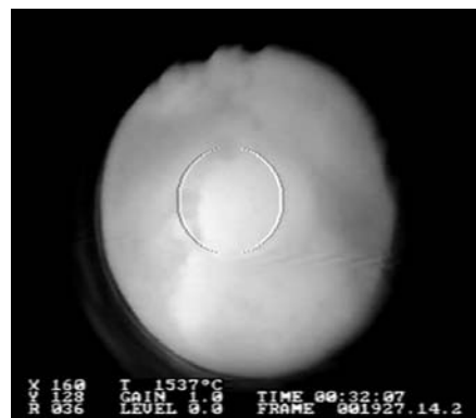
Fig. 6. Video image of the melt surface during the liquidus temperature measurements
