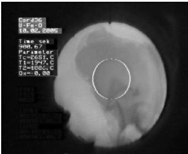
Fig. 3.2. Videoframe of the metallic melt surface
