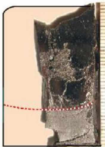
Fig. 3.7. Longitudinal section of the ingot from CORD36
