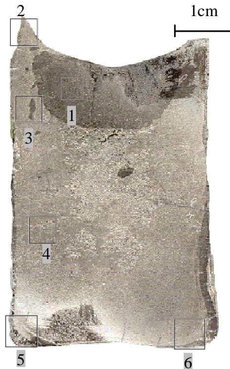
Fig. 3.51. Axial cut of the ingot from CORD39 (cooled from ~2520°C) with regions marked for SEM/EDX analysis
