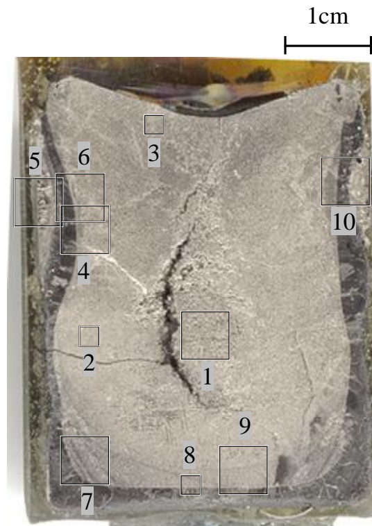
Fig. 3.34. Axial cut of the ingot from CORD35 (cooled from 2120°C) with regions marked for SEM/EDX examination
