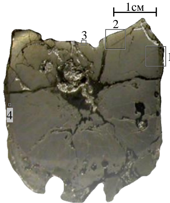
Fig. 7. Longitudinal section of the ingot from CORD46 with regions marked for SEM/EDX analysis
