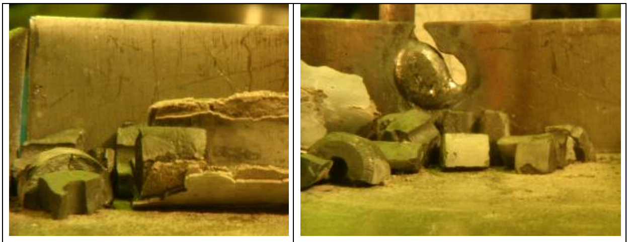
Fig. 7. Temperature history and hydrogen production rate for the test 55. Appearance and fuel fragments of the simulator 55 after the test. (300 \mu m and quench at 1400 ^{\circ} C).
