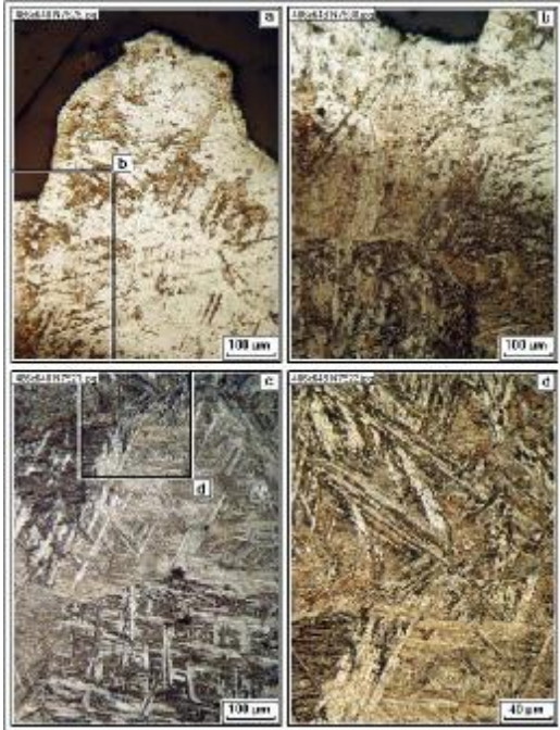
Fig. 1.48 – Steel microstructure near the top surface, area (A)
