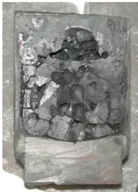
Fig. 2.12 – Longitudinal section of the specimen and corium ingot
