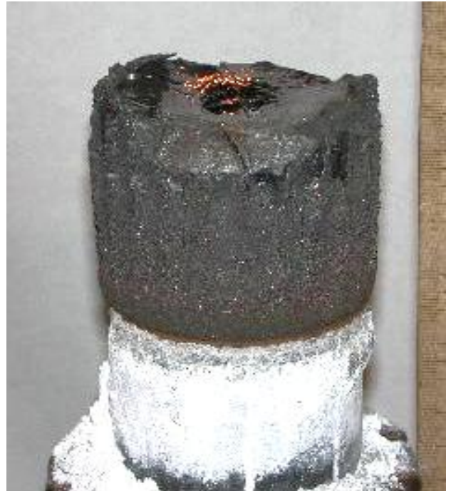
Fig. 1.11. Corium ingot on the steel specimen after the crucible disassembly
