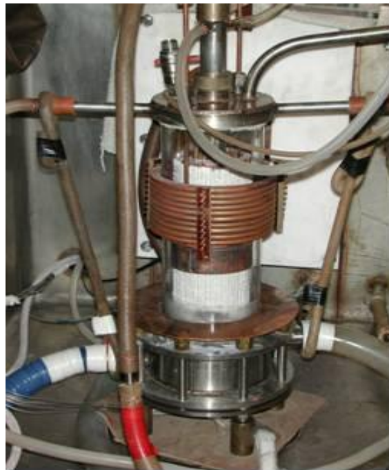
Fig. 1.2. IMCC furnace before the test
