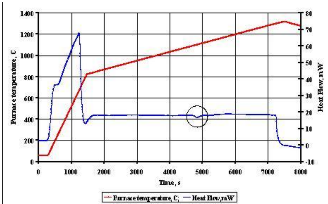
Fig. 2.26. DTA curve during the MC7 sample heating
