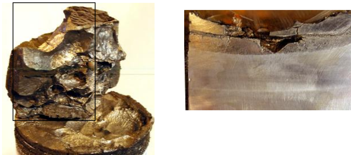
Fig. 2.1.3 – Template cut from the oxidic ingot, and the steel specimen longitudinal section
