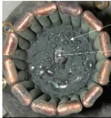
Fig. 4. Corium ingot in the cold crucible in MC5
