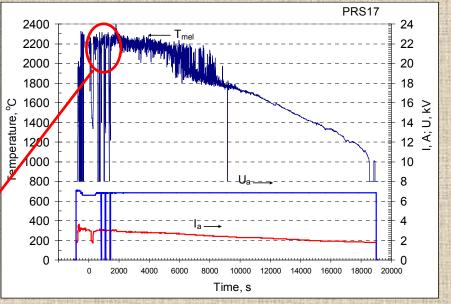
From 1894 s, the pool was pulled out from inductor at 9 mm/h for 4.8 hours. This has ensured close to equilibrium crystallization and the eutectic liquid displacement into the ingot upper part
