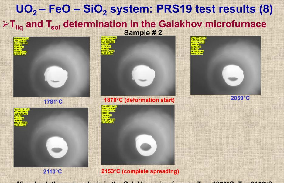
✓Visual polythermal analysis in the Galakhov microfurnace T<sub>sol</sub>= 1870°C; T<sub>liq</sub>=2150°C
