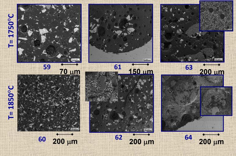
✓ In GPRS 59,60,61 microstructures typical of MG are absent
