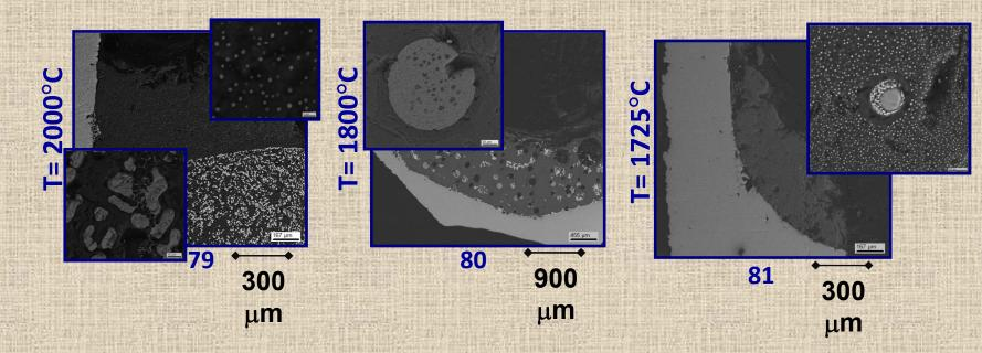
✓ In GPRS 81 microstructures typical of MG are absent
