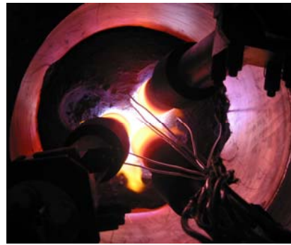
THE PREPARATION TEST WITH ELECTRICAL MELT HEATER AT DIRECT CURRENT OPERATION
