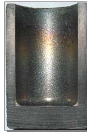
Graphite crucible coated with metallic zirconium
