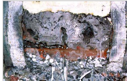
1-D INTERACTION (SIDEWALL MADE FROM MGO) TRAP LINING WITH MORTAR (WITHOUT PEBBLES)
