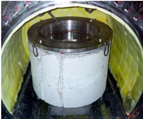
THE TEST SECTION ASSEMBLED WITH LOWER HEAD MODEL AND ELECTRICAL MELT HEATER
