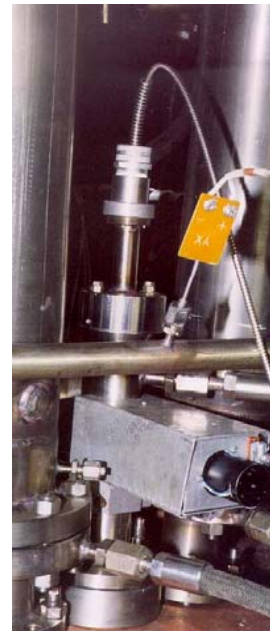
SENSOR MOUNTING ON THE EMF LID
