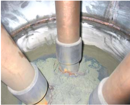
THE PREPARATION TESTS WITH ELECTRICAL MELT HEATER AT ALTERNATING CURRENT OPERATION
