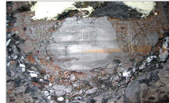
1-D INTERACTION (SIDEWALL MADE FROM MGO) TRAP LINING WITH MORTAR (WITHOUT PEBBLES)
