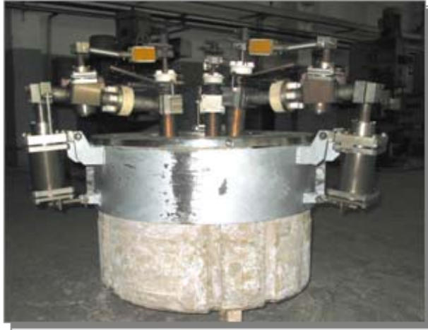
THE TEST SECTION ASSEMBLED WITH LOWER HEAD MODEL AND ELECTRICAL MELT HEATER
