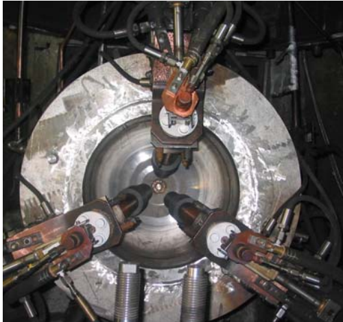
THE TEST SECTION ASSEMBLED WITH LOWER HEAD MODEL AND ELECTRICAL MELT HEATER
