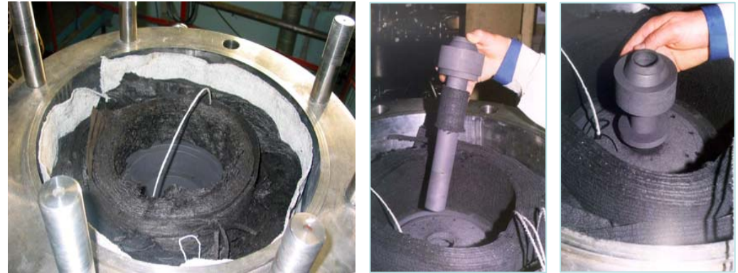
STAGE OF EMF ASSEMBLY AND PROCEDURES ON INSTALLATION OF SENSOR STRUCTURAL ELEMENTS IN THE EMF CRUCIBLE.
