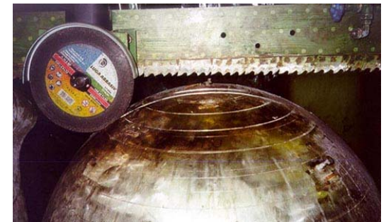
CUTTING OF THE LOWER HEAD
