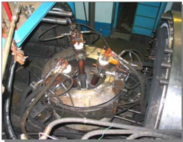
THE LOWER HEAD MODEL WITH ELECTRICAL MELT HEATER ARE LOCATED IN MR OF LAVA-B FACILITY
