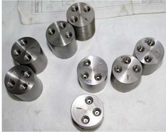
b) Blanks of RPV steel samples
