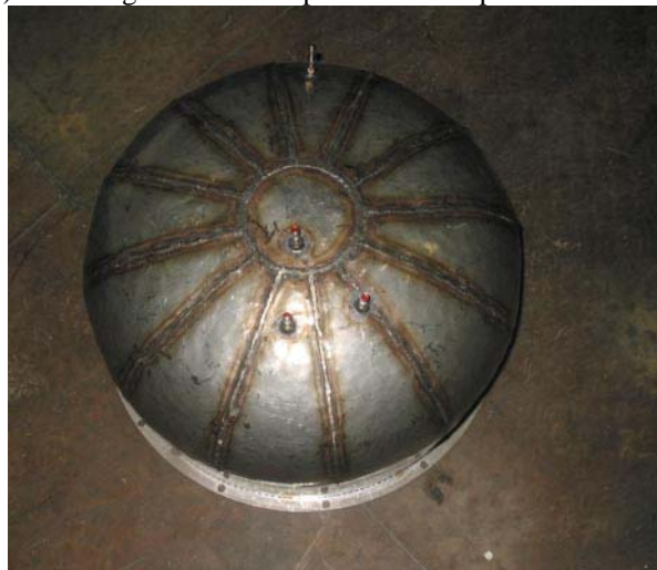
c) Protective steel screen on the external surface of RPV model
