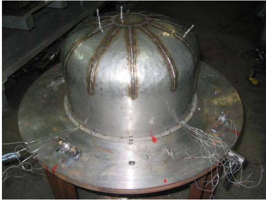
d) Routing of thermocouple wires
