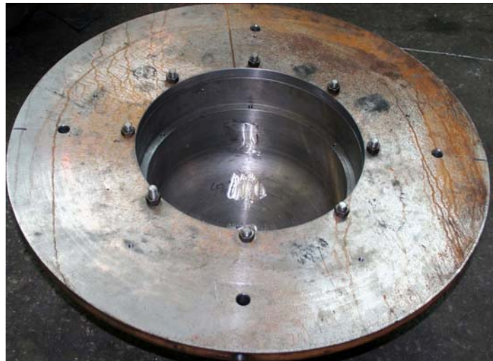
f) RPV model with a flange assembled
