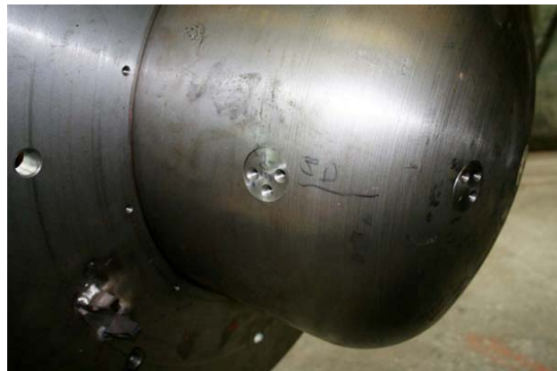
d) View of RPV steel samples from the outer site of RPV model
