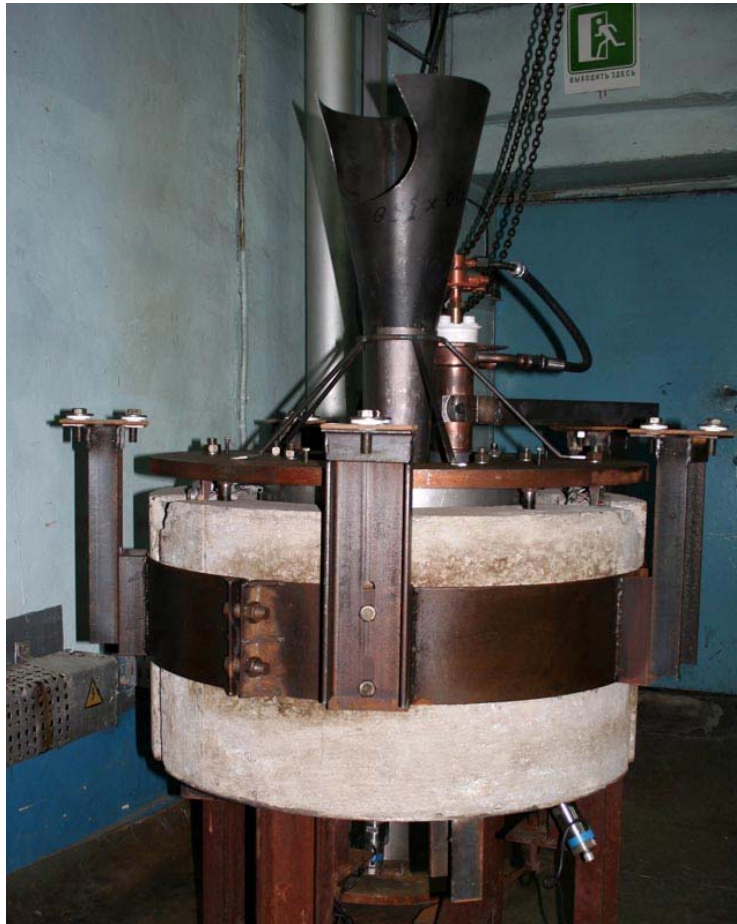
f) Mounting of the RPV model on the concrete base
