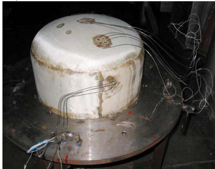
b) Mounting of thermocouples in the samples of RPV steel
