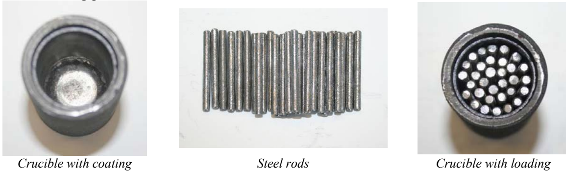
Figure A2.1.12 – Stages of experimental assembly preparation
