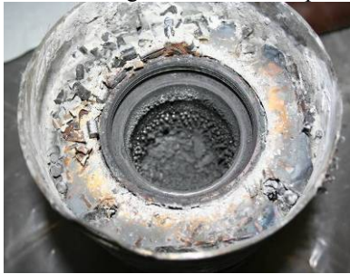
Figure A2.2.33 - Internal surface of the composite graphite outer electrode nozzle bottom and burden in the vessel after removal of a burden part
