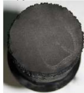
Figure A2.2.13 - Graphite nozzle of the internal electrode after the test. Top view
