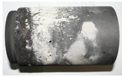
Figure A2.2.34 - Outer surface of the composite graphite outer electrode nozzle top after the test
