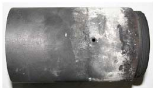
Figure A2.2.13 - Graphite nozzle of the internal electrode after the test. Top view
