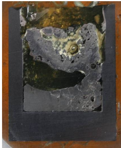
Figure A2.1.6 – Section of the cut surface, Test W - 78.
