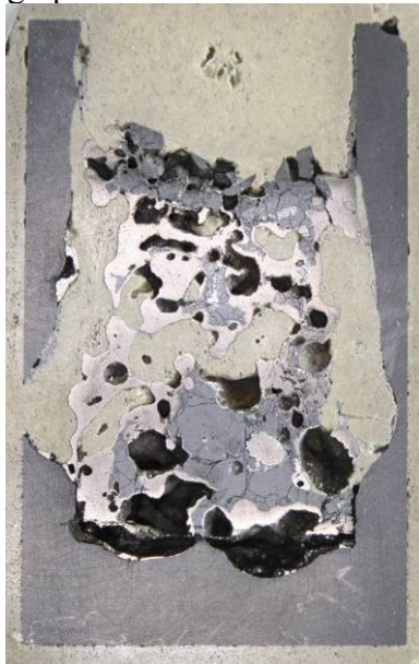
Figure A2.1.2– Surface of crucible cut after Test W-75
