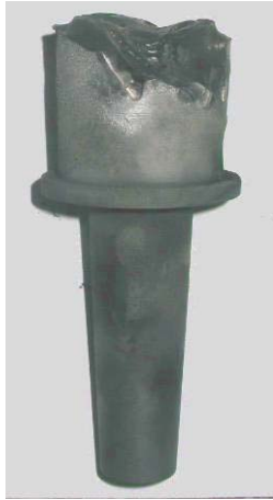
Figure A2.5.37 – Appearance of a nozzle of inner electrode after test (20.11.2008)
