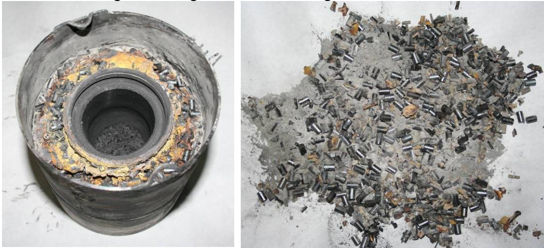
Figure A2.3.5 – Non melted part of loading in the top of the experimental cell Experimental cell has been cut by an abrasive disk in diametrical section, for material fixing before cutting the assemblage has been filled in with molten sulfurs (Figure A2.3.6).
