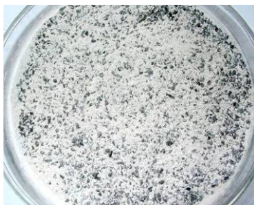
Mixture of UO_2 chips and ZrO_2 powder
