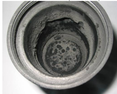
Figure A2.5.39 – State of inner surface of the nozzle of outer electrode after test (20.11.2008)
