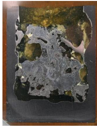
Figure A2.1.4 – Section of the cut surface, Test W 76
