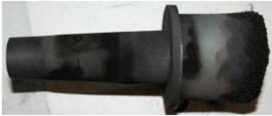
Figure A2.2.12 - Graphite nozzle of the internal electrode after the test. Side view
