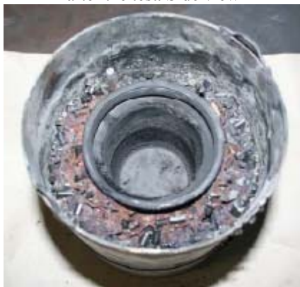
Figure A2.2.14 - Internal surface of the composite graphite outer electrode nozzle bottom and burden in the vessel after removal of a burden part
