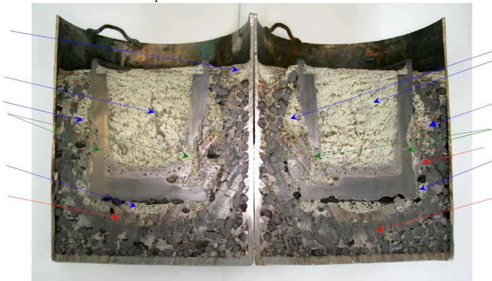
Blue arrows – sulfur, red arrows – melt; green arrows – points of through damage of nozzles
