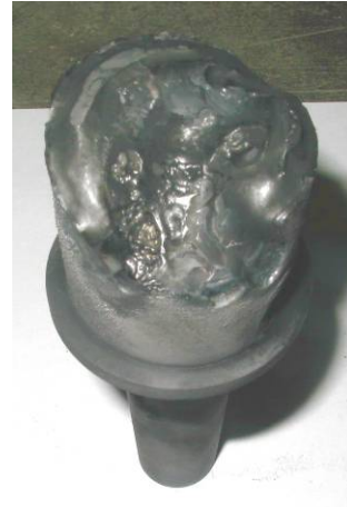
Figure A2.5.37 – Appearance of a nozzle of inner electrode after test (20.11.2008)
