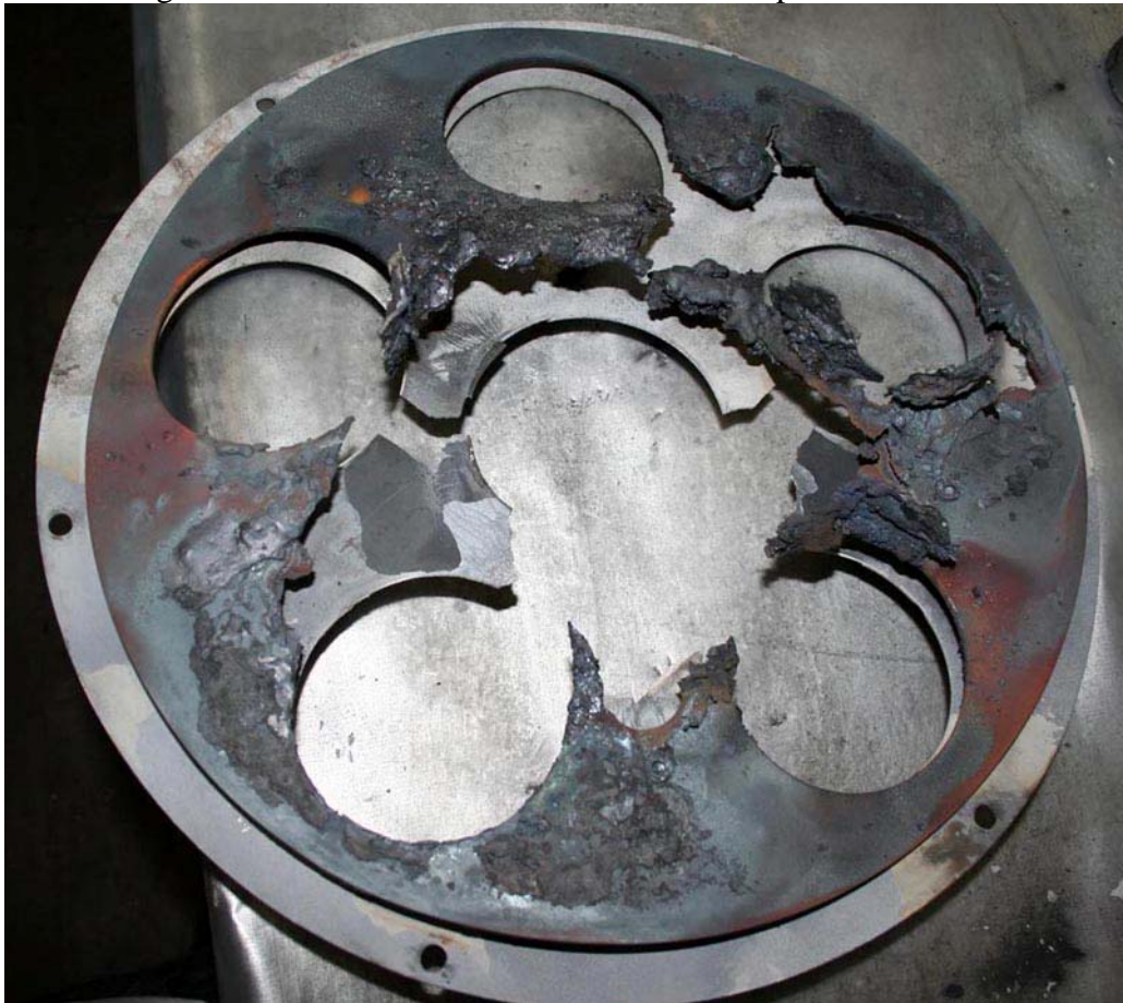
Fig. 2 - Tantalum screen with additional steel plate after test (view from the site of steel plate)
