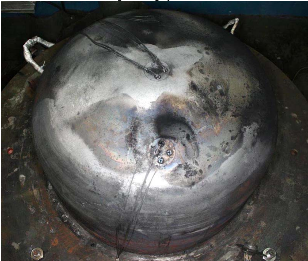
Fig 6 – View of RPV model outer surface (graphite felt has been removed)
