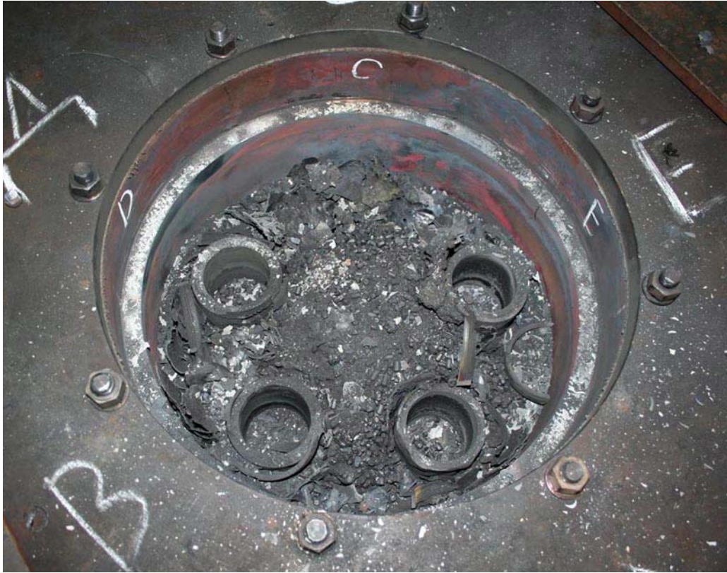
Fig. 3 – View of test section after test (thermal screen and top parts of plasmatrons have been removed)
