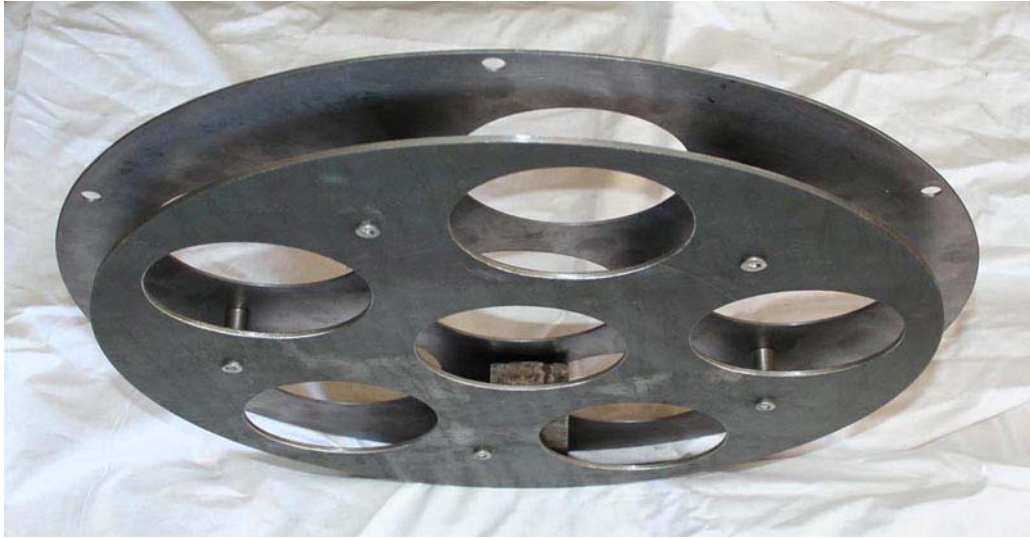
Fig. 1 – Tantalum screen with additional steel plate before test
