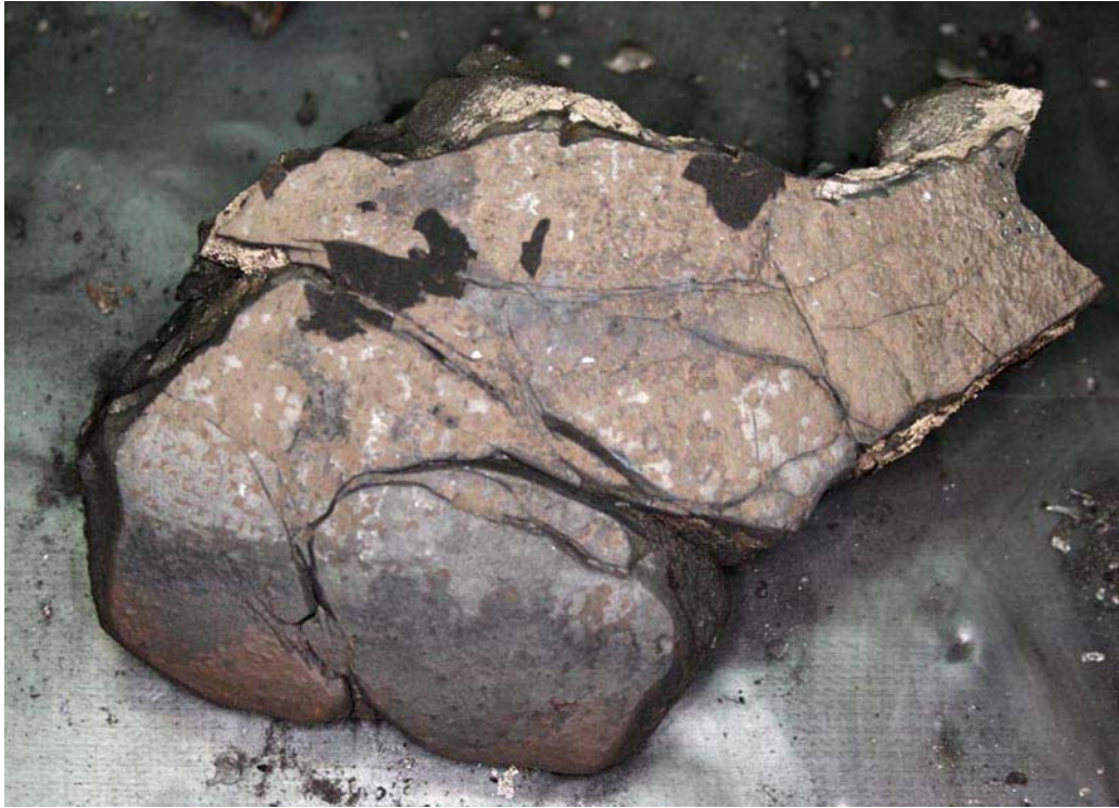
Fig. 7 – Fragment of corium ingot (view from the surface contacted with RPV model wall)
