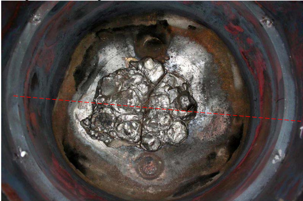
Fig. 8 – View of RPV model with corium ingot adhered to the RPV model wall (will be cut along the red line)
