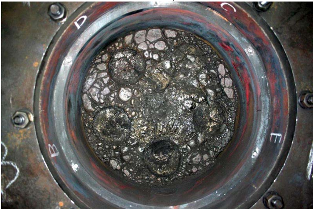
Fig. 4 – View of test section after test (fragmented debris bed and plasmatrons nozzles have been removed)
