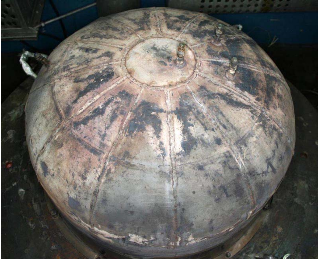
Fig. 5 – View of stainless steel housing outside graphite felt on the outer surface of RPV model
