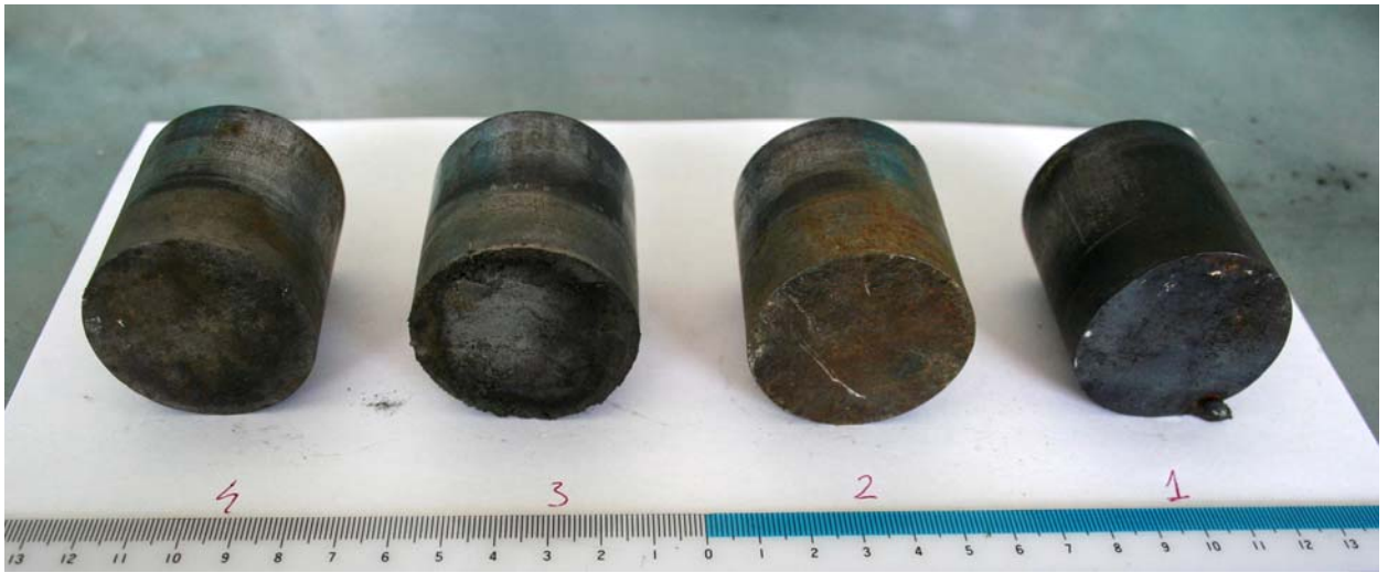
Fig. 10 – Samples of RPV steel extracted from carbon steel matrix (Numbers correspond to the scheme below. Surface of steel in interface "corium/steel" is fused especially in the central zone (sample #3))
