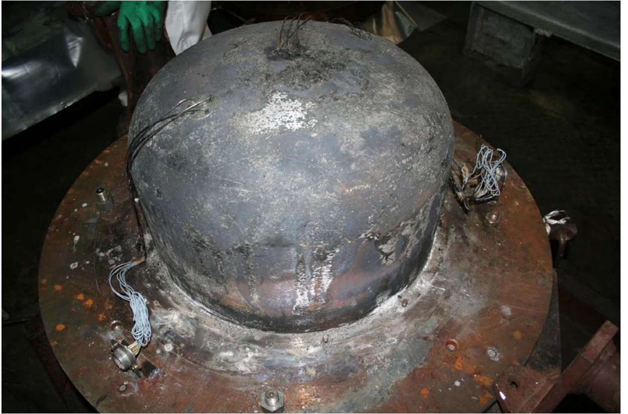
Fig. 3 – Outer surface of RPV model after glass cloth removal
