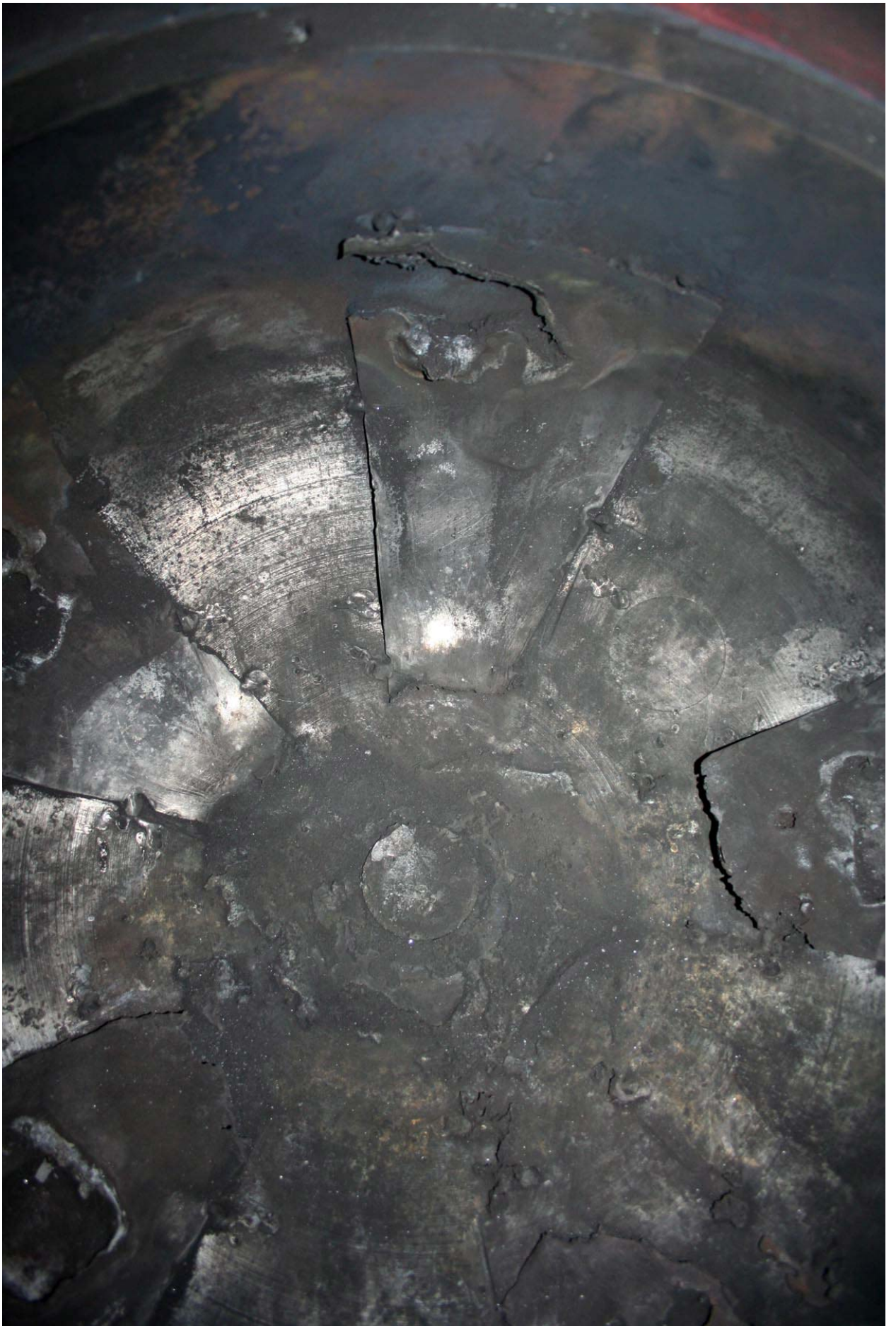
Fig. 4 – Inner surface of RPV model after corium ingot removal
