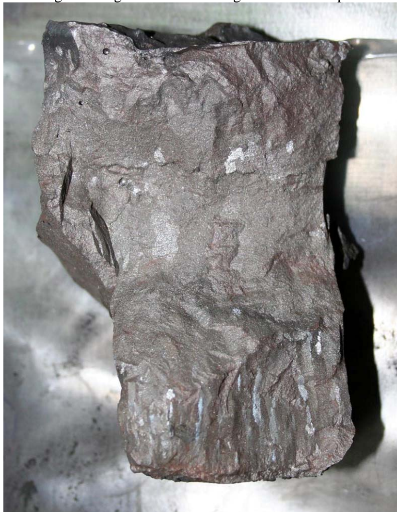
Fig. 9 – Fragment of corium ingot from central part (sample for research)
