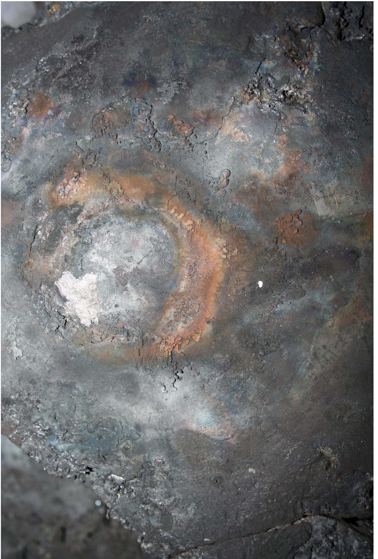
Fig. 7 – Top view of corium ingot (central part)
