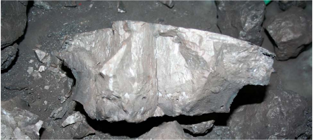
Fig. 8 – Fragment of corium ingot from central part
