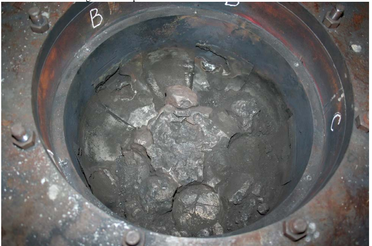
Fig. 2 – Solidified corium in RPV model after particulate debris removal
