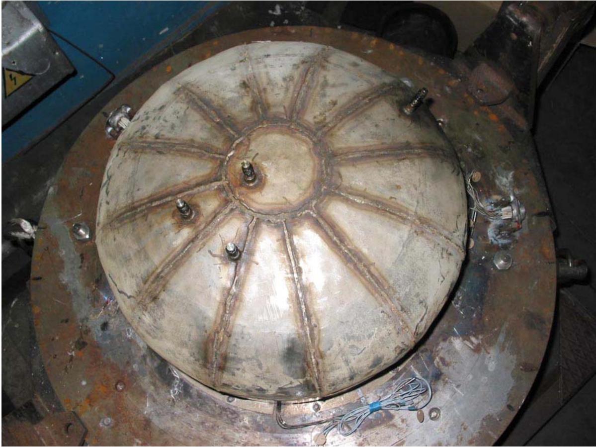
Fig.5 – Outer surface of RPV model covered with glass cloth and SS sheet
