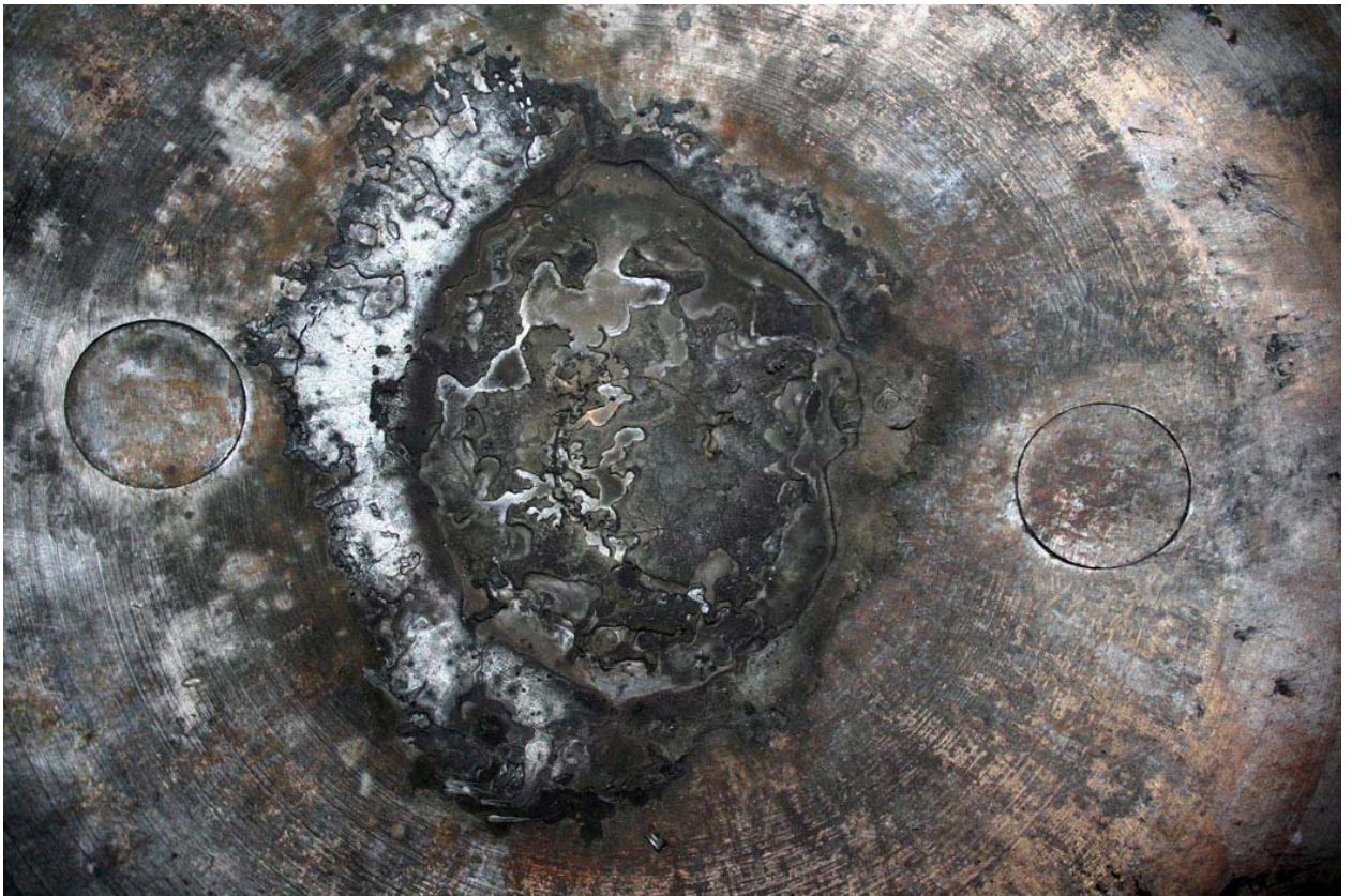
Fig. 17 - Inner surface of RPV model after corium ingot removal (close-up view of fused zone)
