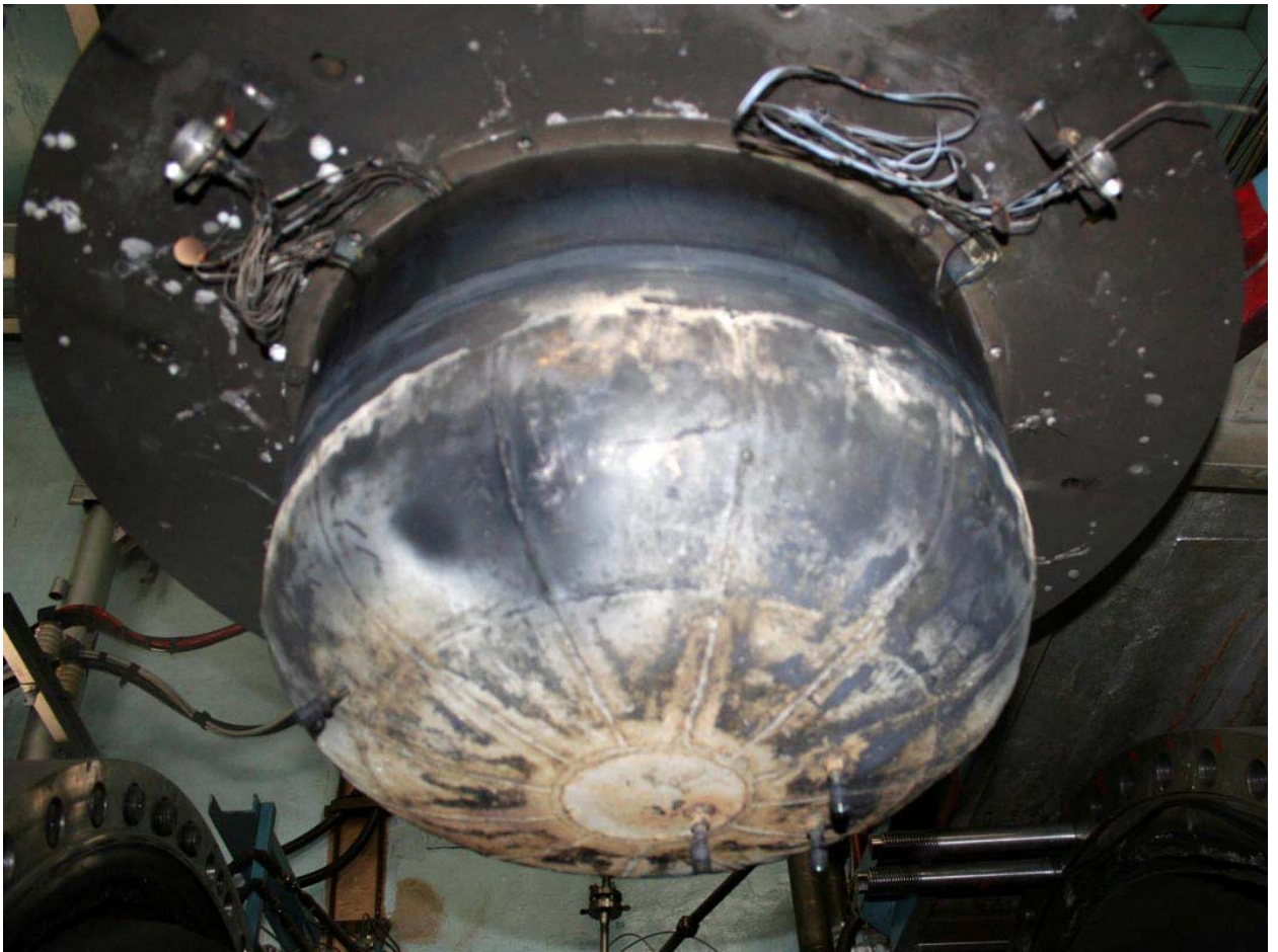
Fig. 7 SS sheet outside of RPV model after test
