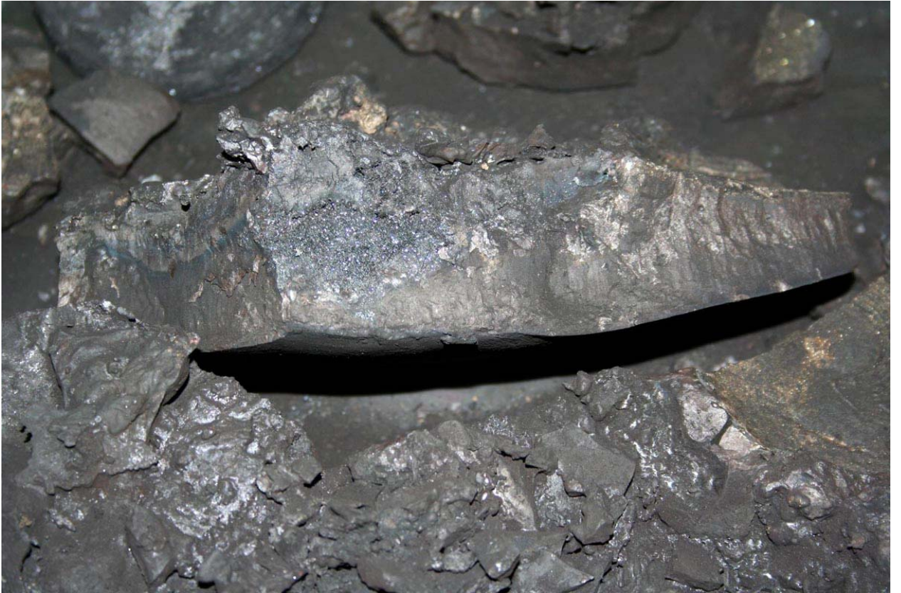
Fig. 19 – Fragment of corium ingot breaking surface
