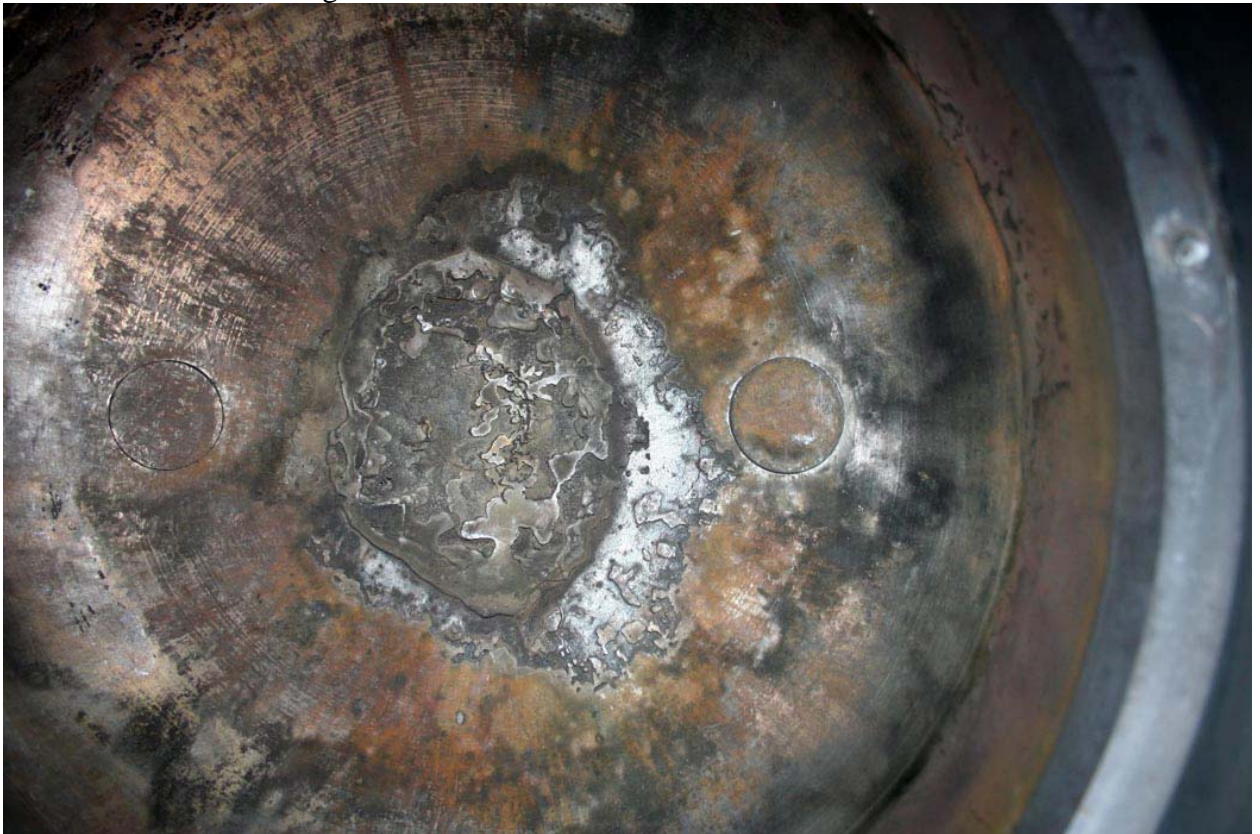
Fig. 16 – Inner surface of RPV model after corium ingot removal
