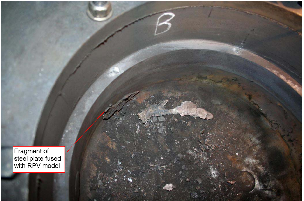
Fig. 15 – View of RPV model after corium removal
