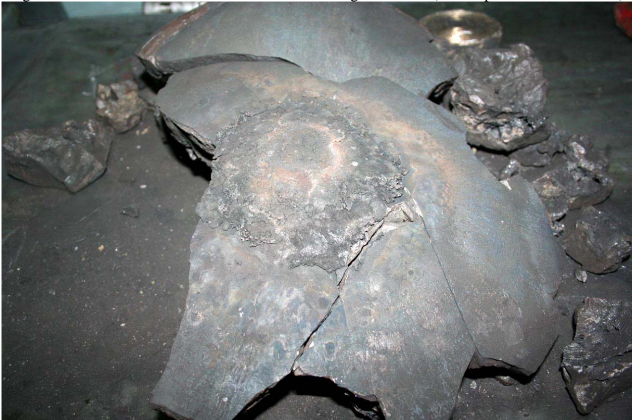
Fig. 18 – Upper view of corium ingot (from the site of contact with RPV bottom)
