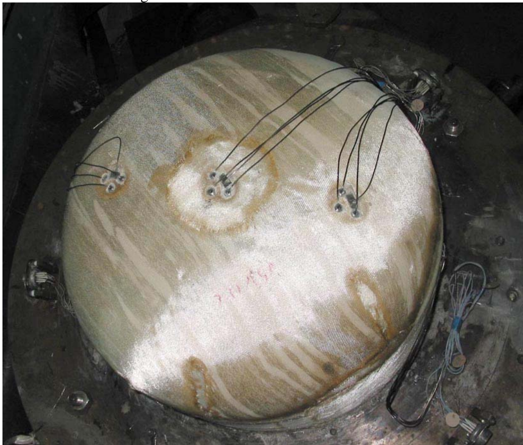
Fig. 4 – Initial outer surface of RPV model lined with glass cloth
