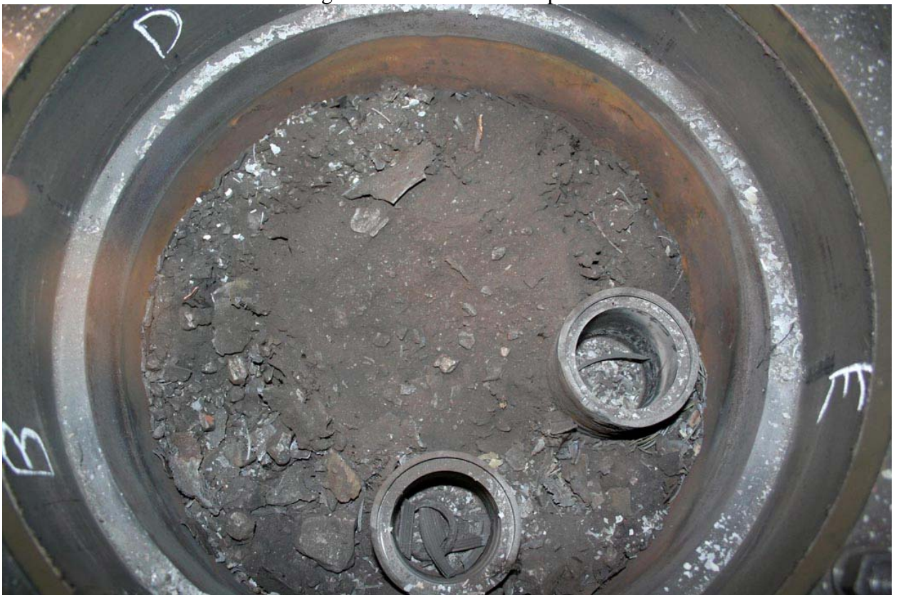
Fig. 12 - RPV model with corium after steel plate removal
