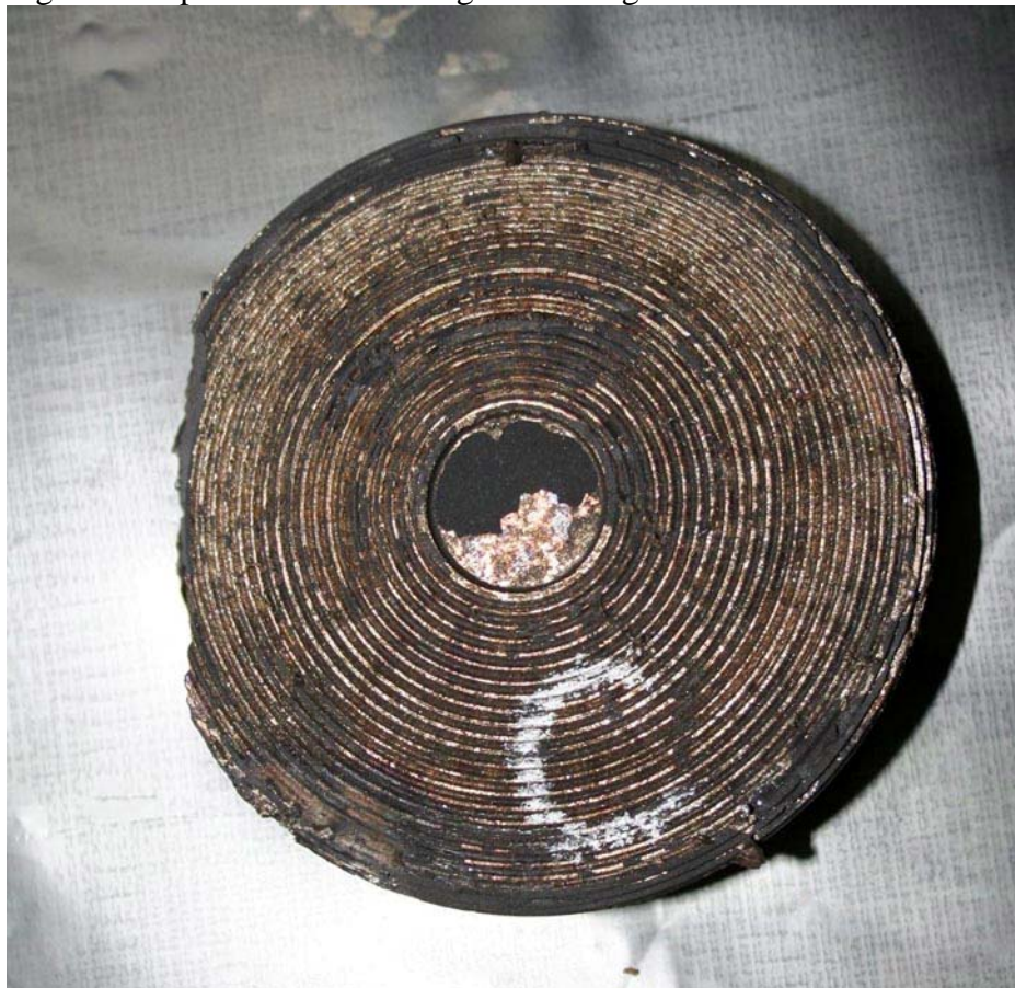
Fig. 14 – Upper view of plasmatron nozzle with remains of protective coating
