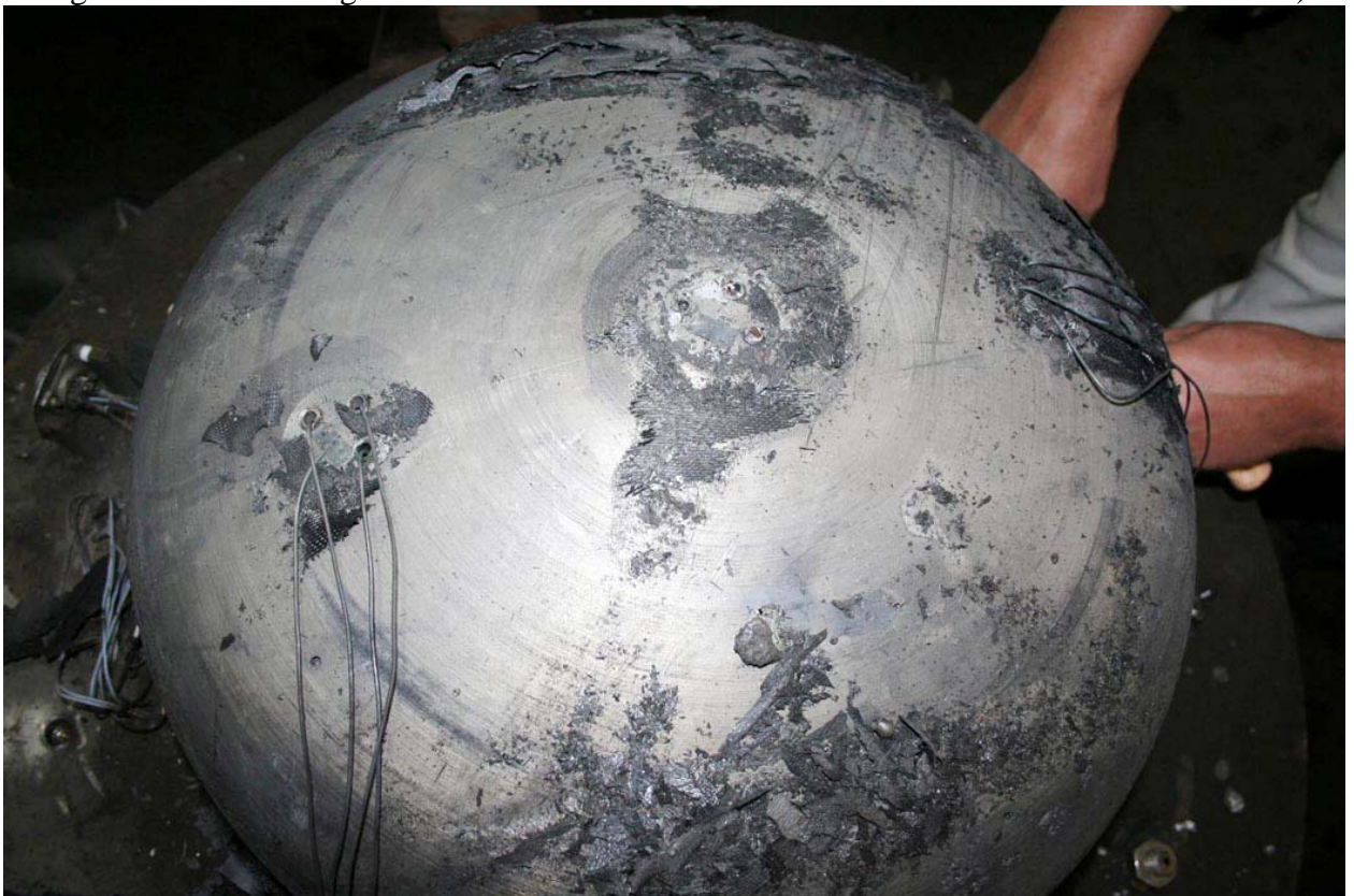
Fig. 22 – Outer surface of RPV model after thermal insulation removal
