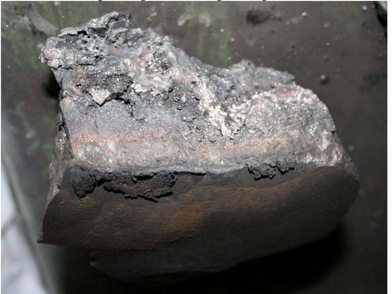
Fig. 20 – Fragment of corium ingot breaking surface
